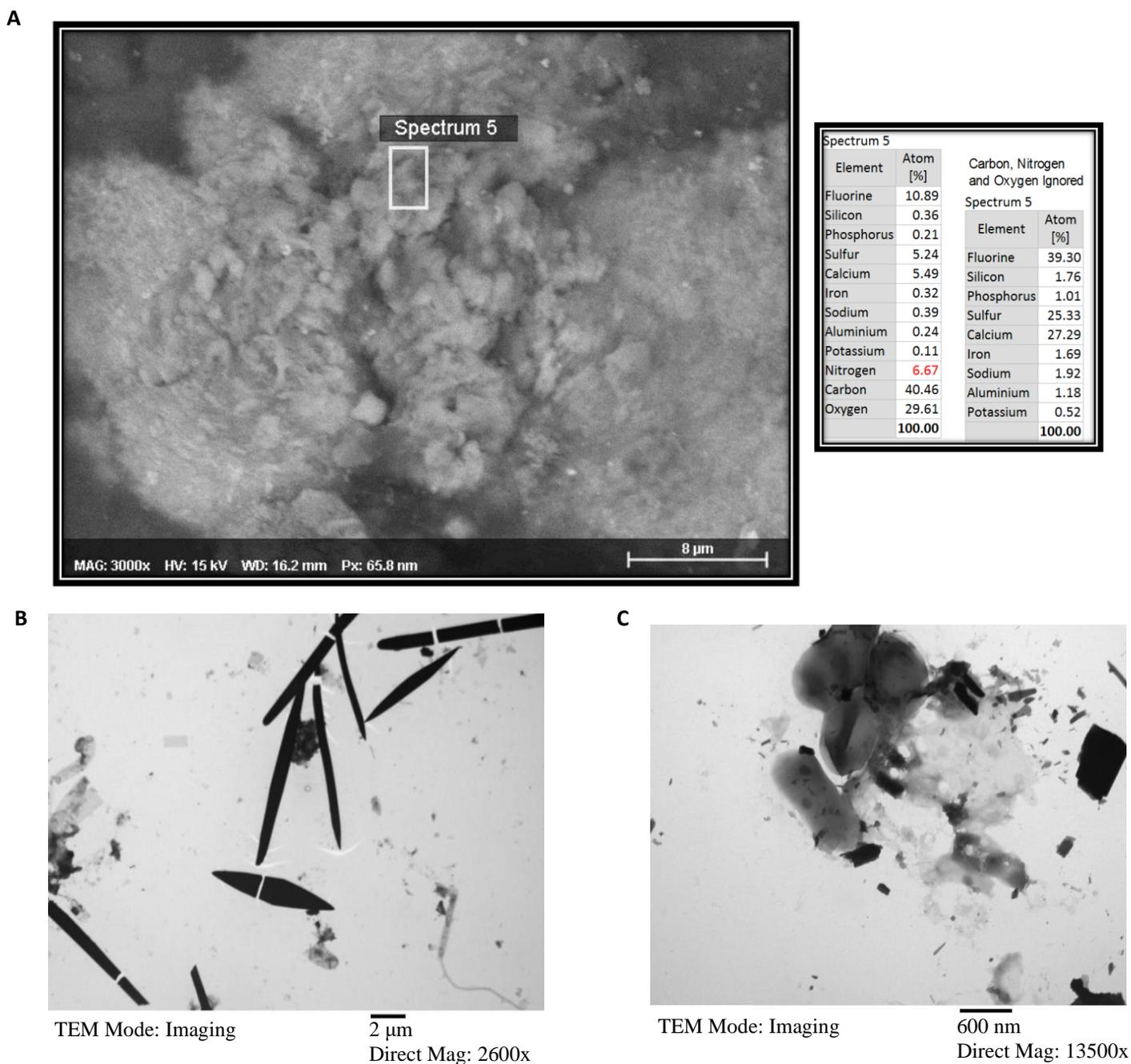
**Figure 5.** Representative micrographs and microscopy results. (A) shows a representative scanning electron microscope image and its accompanying EDX table for spectrum 5. (B) and (C) are transmission electron microscope images of inorganic crystalline calcium sulfate, an unexpected inorganic scalant that was encountered throughout the foulant cake layer.
