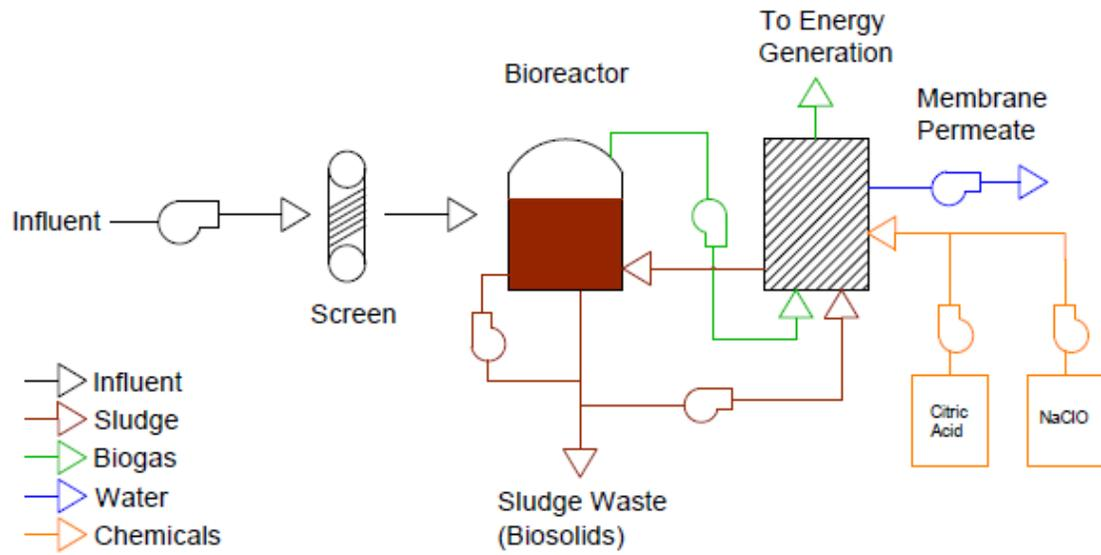
**Figure 1.** Zoomed in schematic on the bioreactor and the membrane tank. The membrane cleaning sequence is clearly elucidated as shown by the chemical addition to the membrane module section only.
