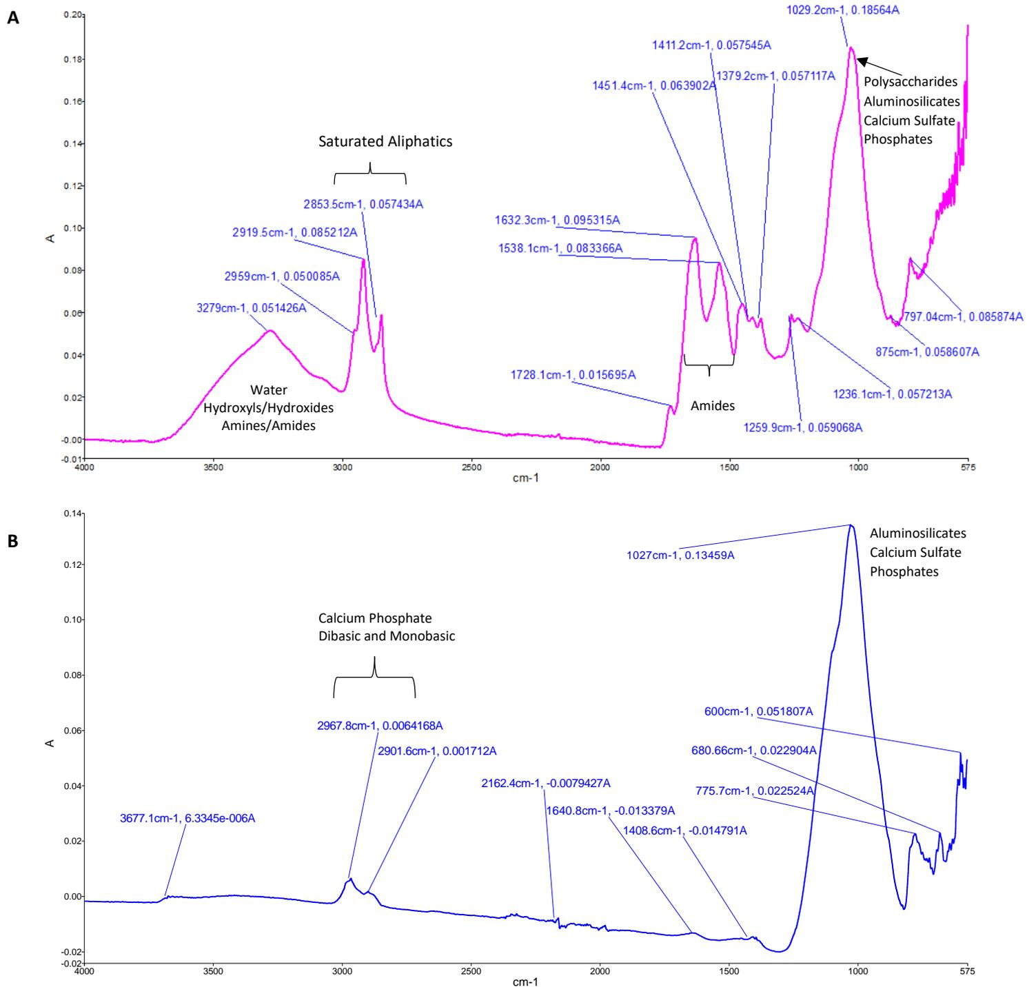
**Figure 4.** Fourier Transform Infrared (FTIR) Spectroscopy Spectra of dehydrated foulant from the cake layer (A) and foulant after ignition at 450°C for 8 hours to combust the organic materials present and leave only inorganics (B).
