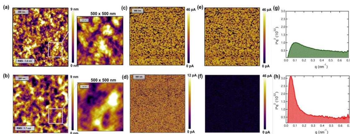
**Fig. 3** Normalized AFM topography images of (a) 1% LMWF PM6:Y6 and (b) 52% LMWF PM6:Y6 blends. photoconductive AFM images taken at 0V bias and under white light illumination of (c) 1% LMWF PM6:Y6 and (d) 52% LMWF PM6:Y6 blends. The corresponding normalized photoconductive AFM images of (e) 1% LMWF PM6:Y6 and (f) 52% LMWF PM6:Y6 blends. Lorentz corrected and circularly averaged RSoXS profiles of the (g) 1% LMWF PM6:Y6 and (h) 52% LMWF PM6:Y6 blend systems.
