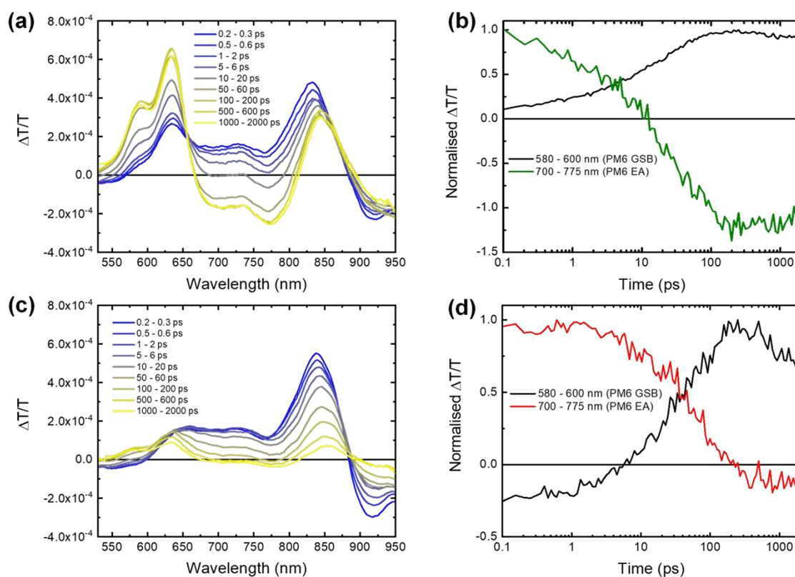
**Fig. 5** Visible region TA spectra and fitted kinetics of the PM6:Y6 (a,b) 1% LMWF blend (pump: 800 nm and fluence:  $0.45 \mu\text{J cm}^{-2}$ ) and (c,d) 52% LMWF blend (pump: 800 nm and fluence:  $0.50 \mu\text{J cm}^{-2}$ ).
