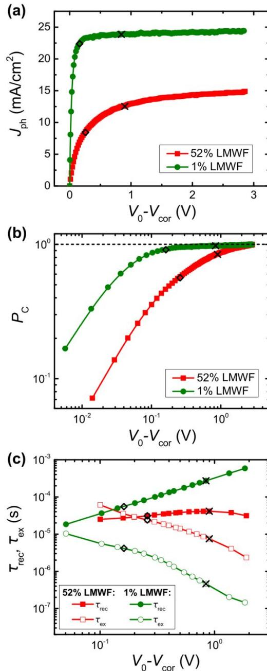
**Fig. 6** (a) Photocurrent  $J_{\text{ph}}$  and (b) collection probability  $P_C$  of the 1% and 52% LMWF PM6:Y6 batches. (c) Average extraction time  $\tau_{\text{ex}}$  and charge carrier lifetime  $\tau_{\text{rec}}$  of the two batches.
