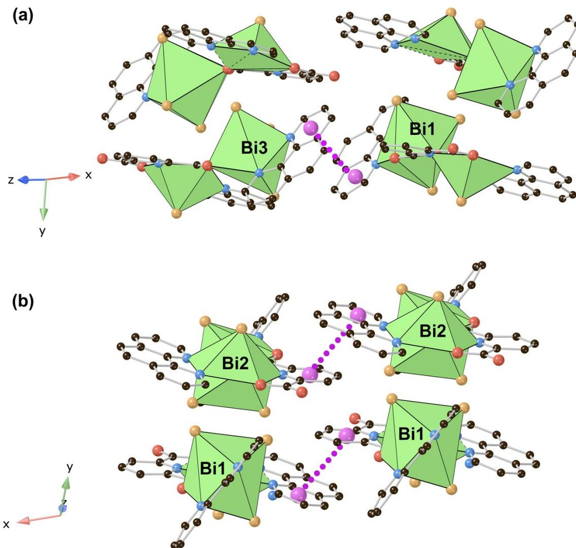
**Fig. 2** Polyhedral representation of **1** showing  $\pi$ - $\pi$  stacking interactions (purple dashed lines) between (a) two phenanthroline from adjacent Bi1, Bi2 and Bi3, Bi4 tetramers and (b) phen and PDC from two Bi1, Bi2 tetramers. Green polyhedra, red, orange, blue, and black spheres represent bismuth, oxygen, chlorine, nitrogen, and carbon atoms, respectively. Purple spheres represent ring centroids. Hydrogen atoms and acetonitrile solvent molecules have been omitted for clarity.
