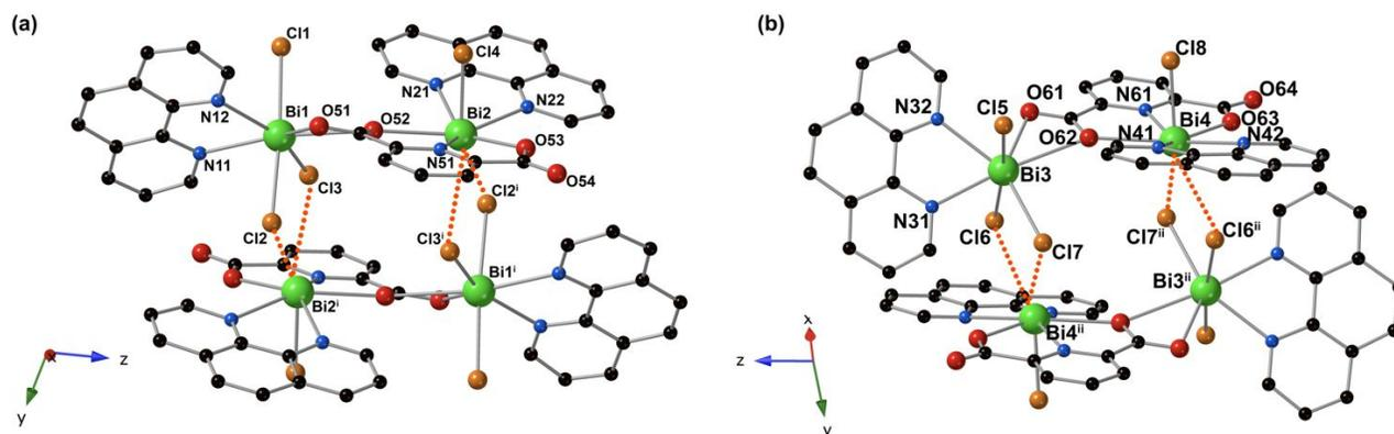
**Fig. 1.** Illustration of the two unique tetrameric units in **1** which are built from (a) Bi1 and Bi2 and (b) Bi3 and Bi4. Green, red, orange, blue, and black spheres represent bismuth, oxygen, chlorine, nitrogen, and carbon atoms, respectively. Dotted orange lines denote long Bi...Cl interactions. Hydrogen atoms and acetonitrile solvent molecules have been omitted for clarity. Symmetry operators: (i)  $2 - x, 1 - y, 1 - z$ ; (ii)  $1 - x, 1 - y, -z$ .
