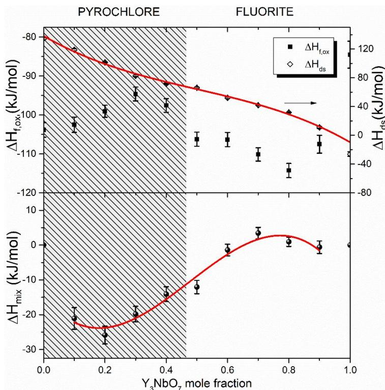
Figure 4 Enthalpies of drop solution and formation from binary oxides (top), enthalpies of mixing (bottom) of  $Y_3NbO_7$  -  $Y_2Ti_2O_7$  solid solutions. The error is two standard deviations of the mean.
