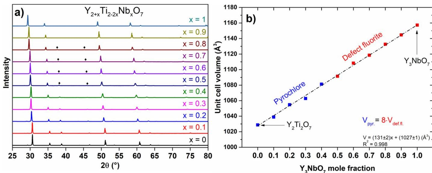
Figure 2 a) X-ray diffractograms of synthesized  $\text{Y}_{2+x}\text{Ti}_{2-2x}\text{Nb}_x\text{O}_7$  solid solutions. Black diamonds mark the reflections around 38° and 47° which correspond to additional pyrochlore ordering, b) normalized volume of the unit cell of  $\text{Y}_{2+x}\text{Ti}_{2-2x}\text{Nb}_x\text{O}_7$ .
