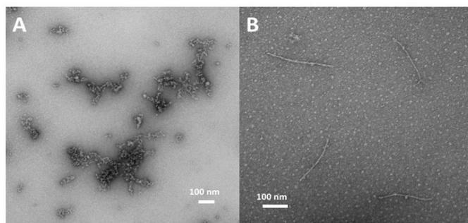
**Fig. 3** TEM images of **1-closed** after 254 nm irradiation in methanol, evaporation, and redissolution in water (10 mM): (A) without sonication after 24 h and (B) 10 min after sonication (20% amp., 5 min, pulsed 10 s on, 5 s off). TEM images were recorded after diluting in water (1 mM) and evaporating onto a carbon-coated copper grid with 2% aq. uranyl acetate as a negative stain.
