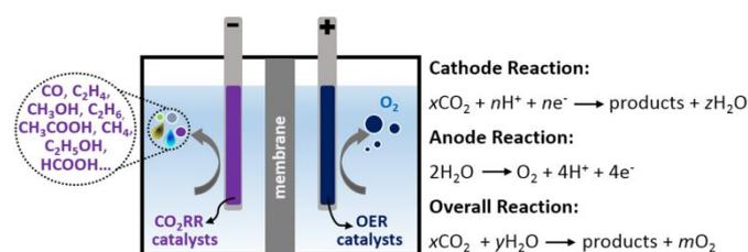
Fig. 1 Illustration of a traditional CO<sub>2</sub> reduction electrolyzer.
