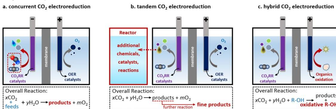
**Fig. 3** Three innovative strategies of (a) concurrent CO<sub>2</sub> electroreduction, (b) tandem CO<sub>2</sub> electroreduction, and (c) hybrid CO<sub>2</sub> electroreduction for nonconventional CO<sub>2</sub>RR.
