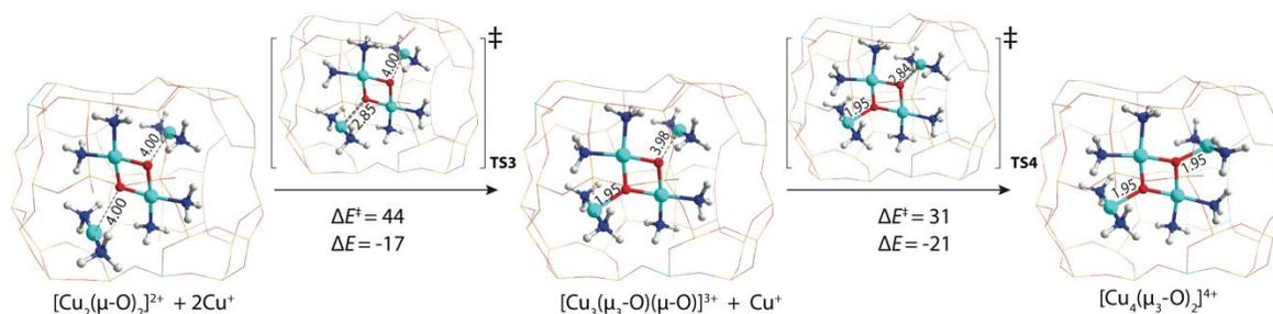
**Fig. 3** Formation of tetranuclear  $[\text{Cu}_4(\mu_3\text{-O})_2]^{4+}$  via the reaction of dimeric  $[\text{Cu}_2(\mu\text{-O})_2]^{2+}$  and an extra pair of  $[\text{Cu}(\text{NH}_3)_2]^+$  confined in one CHA cage. Activation and reaction energies ( $\Delta E^\ddagger$  and  $\Delta E$ ) are given in kJ/mol. Cu–O distances are indicated in Å.
