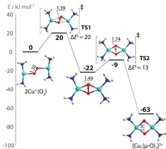
**Fig. 2** Energy profiles for O<sub>2</sub> dissociation and oxidation of two mononuclear [Cu(NH<sub>3</sub>)<sub>2</sub>]<sup>+</sup>. Zeolite frameworks are omitted for clarity. Atomic distances are given in Å.
