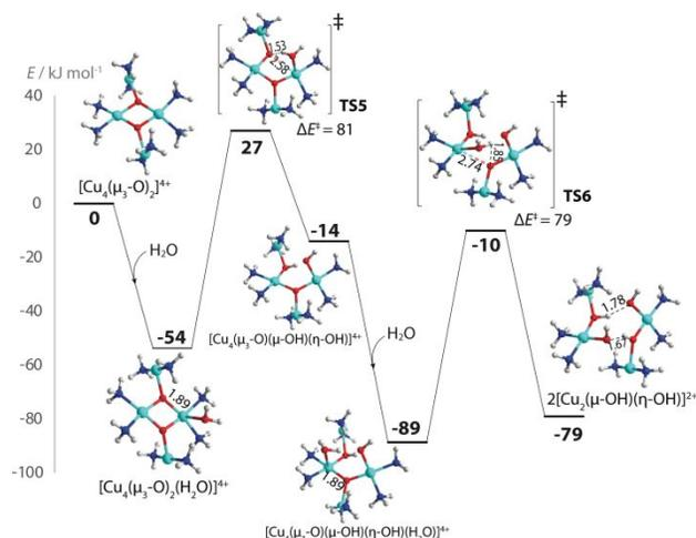
**Fig. 4** Energy profiles for the H<sub>2</sub>O-assisted decomposition of a tetranuclear [Cu<sub>4</sub>(μ<sub>3</sub>-O)<sub>2</sub>]<sup>4+</sup> into two dicopper [Cu<sub>2</sub>(μ-OH)(η-OH)]<sup>2+</sup> sites. Zeolite frameworks are omitted for clarity. Atomic distances are given in Å.
