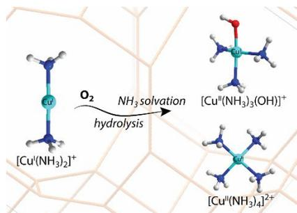
DFT calculations suggest Cu(I) oxidation with O<sub>2</sub> as the sole oxidant plays a major role in oxidation half cycle of standard NH<sub>3</sub>-SCR over Cu-CHA zeolites.
