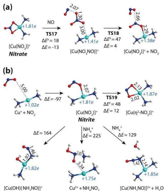
**Fig. 8** Reaction pathways for the conversion of cationic cupric (a) nitrate and (b) nitrite species in CHA cage. Zeolite frameworks are omitted for clarity. Activation and reaction energies ( $\Delta E^\ddagger$  and  $\Delta E$ ) are given in kJ/mol. The Bader charges of Cu are normalized with reference to the bulk CuO (+2.00  $e$ ).
