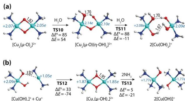
**Fig. 6** (a) H<sub>2</sub>O-assisted decomposition of a dimeric [Cu<sub>2</sub>(μ-O)<sub>2</sub>]<sup>2+</sup> into two mononuclear [Cu(OH)<sub>2</sub>]<sup>+</sup> intermediates; (b) NH<sub>3</sub> solvation assisted formation of two [Cu(OH)]<sup>+</sup> sites from the reaction of [Cu(OH)<sub>2</sub>]<sup>+</sup> and Cu(I) ions. Zeolite frameworks are omitted for clarity. Atomic distances are given in Å. The Bader charges of Cu are normalized with reference to the bulk CuO (+2.00 e).
