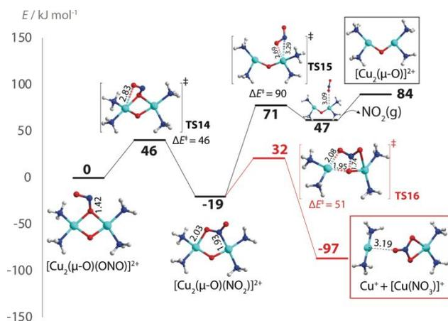
**Fig. 7** Energy profile for the NO-assisted activation of Cu(I) into Cu(II) species in CHA zeolite. Zeolite frameworks are omitted for clarity. Atomic distances are given in Å.
