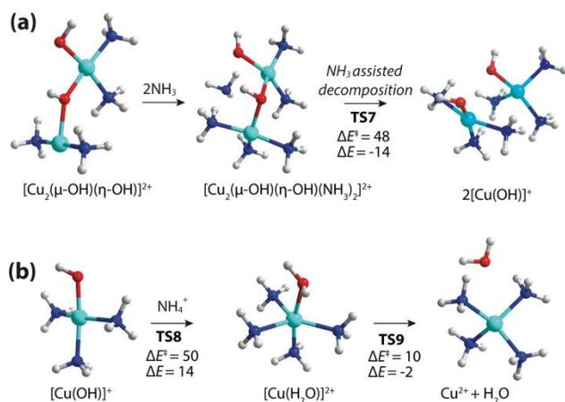
**Fig. 5** (a) NH<sub>3</sub> assisted decomposition of dicopper [Cu<sub>2</sub>(μ-OH)(η-OH)]<sup>2+</sup> into two [Cu(OH)]<sup>+</sup> ions; (b) Formation of Cu<sup>2+</sup> species from the dehydration reaction of [Cu(OH)]<sup>+</sup> and a Brønsted proton (in the form of NH<sub>4</sub><sup>+</sup>). Activation and reaction energies (ΔE<sup>‡</sup> and ΔE) are in kJ/mol. Zeolite frameworks are omitted for clarity.
