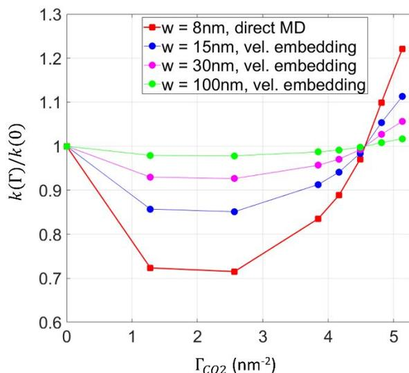
**Fig. 2.** Variation of the decane permeability of calcite slit pores at different  $\text{CO}_2$  adsorption densities  $\Gamma_{\text{CO}_2}$ .
