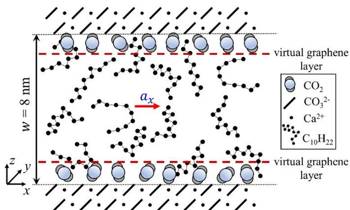
**Fig. 1.** A schematic of the simulation system for studying decane transport through slit calcite pores. Virtual graphene layers (red dashed lines) interacting only with CO<sub>2</sub> confine them near the calcite surface to ensure a well-defined CO<sub>2</sub> adsorption density during simulation.  $z = 0$  corresponds to the uppermost oxygen atom layer of the lower calcite slab.
