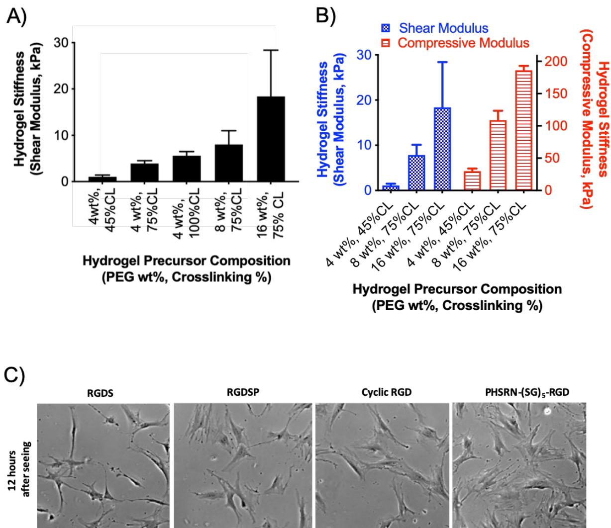
**Figure S2.** Controllable hydrogel substrate stiffness and adhesivity. A,B) Hydrogel stiffness is tunable by changing the polymer concentration (weight percentage) and crosslinking density (total percentage of norbornene arms crosslinked). C) Adhesivity is controlled by changing the identity and concentration of integrin-binding peptides.
