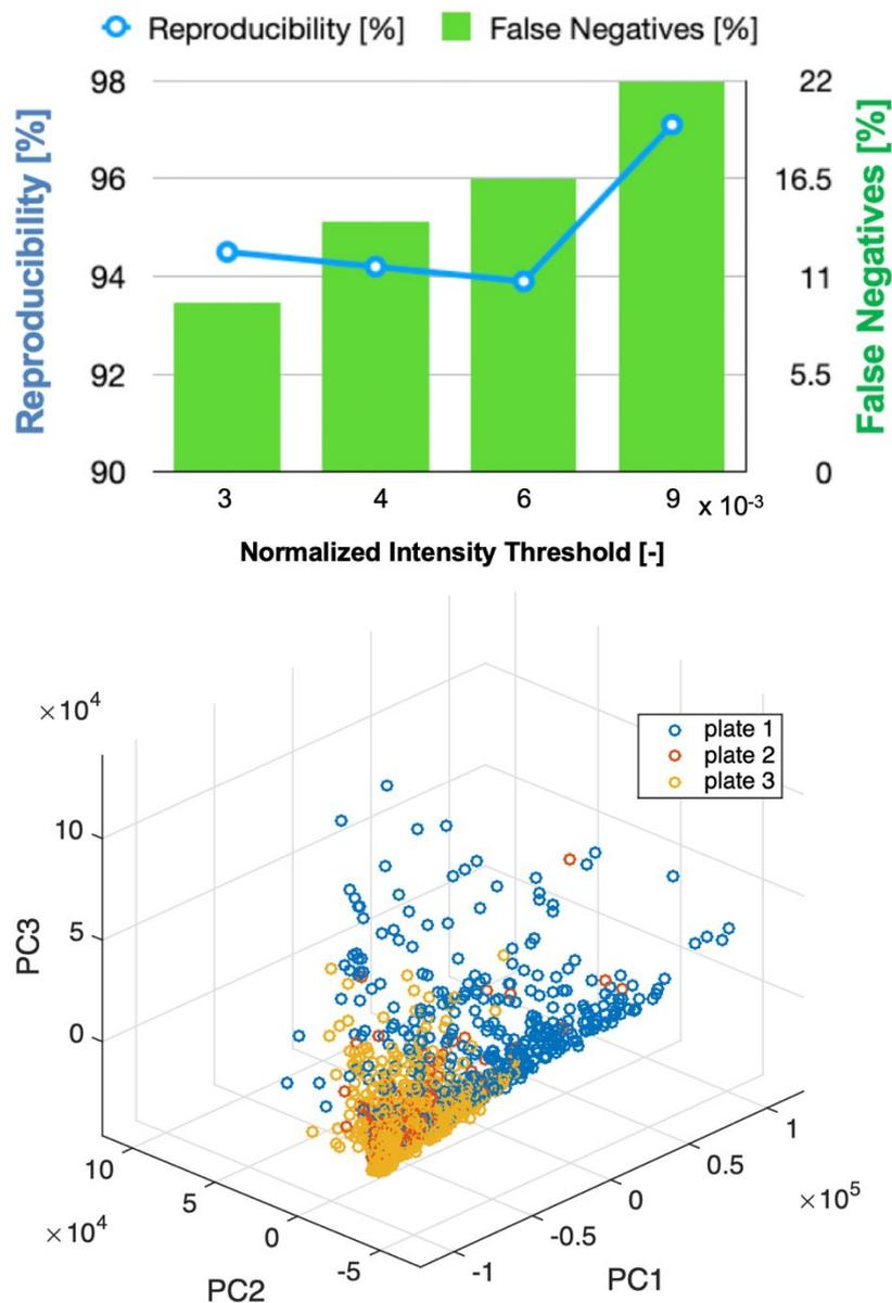
**Figure 10** (Top) Trade-off between repeatability and the rate of false negatives at different normalized intensity threshold for determining yes/no reactions. (Bottom) Coefficients of the first 3 principal components (PC) of the spotted rhodamine spectra in 3 plates over 3 days. The PCs occupy the same space between substrates and suggest that the variability of the MS spectrum is well characterized and consistent in each HTS experiment.
