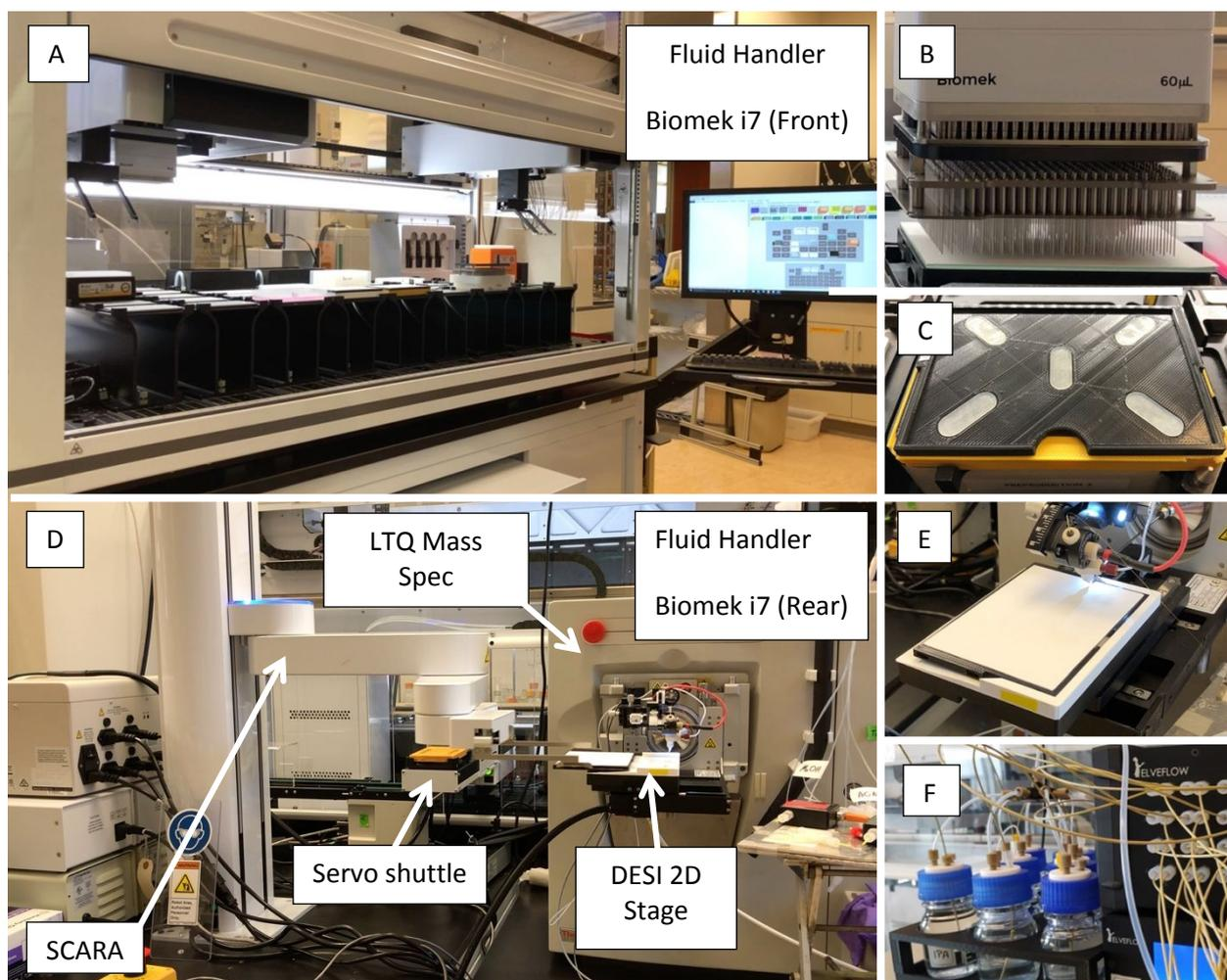
**Figure 2** Photographs showing the key components of the DESI-MS HTS system, including (A) a fluid handling workstation (Biomek i7, Beckman Coulter Inc.) which includes (B) pin tool and (C) a plate holder (C), (D) a SCARA robot (PF3400, Precise Automation Inc.), (E) a DESI-2D imaging stage (DESI 2D, Prosolia Inc.) installed on an LTQ XL mass spectrometer (Thermo Scientific), and (F) a DESI spray solvent delivery system (ElveFlow).
