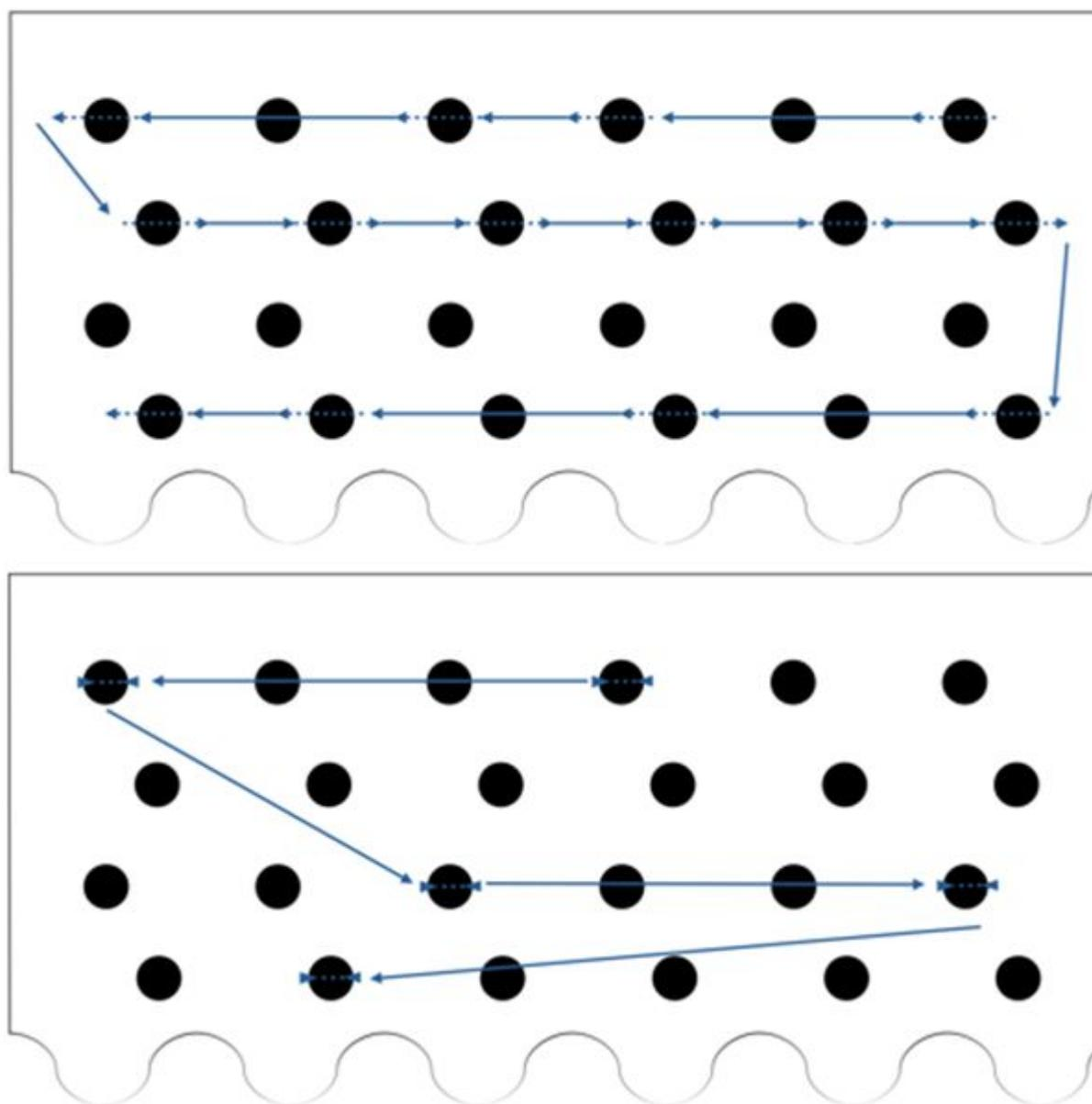
**Figure 11** (Top) Spot-to-spot method of data acquisition. The spots that are skipped represent locations that were not selected for analysis by the user. (Bottom) Example of MS/MS spot-to-spot data acquisition. Data is acquired only from specific locations provided by the user. Since not all reactions produce product, MS/MS data is typically acquired from far fewer spots.
