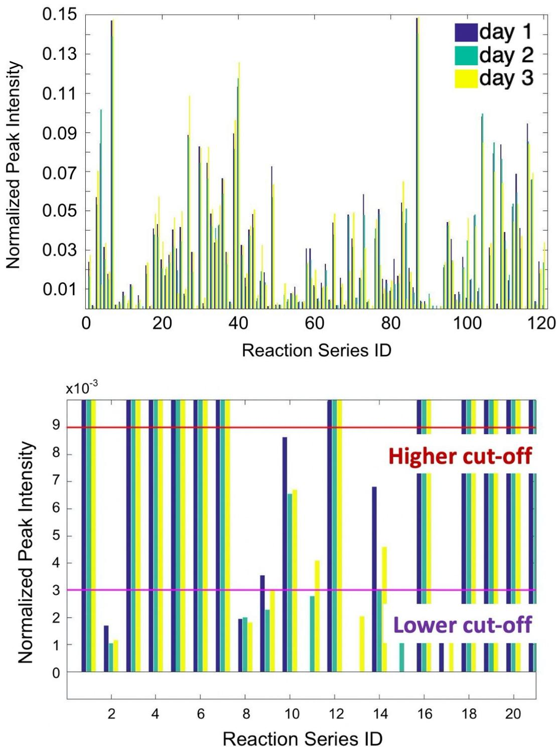
**Figure 9** (Top) Normalized MS intensity of 120 reaction products performed in the 3-by-8-hour case study. (Bottom) Zoomed-in plot of the first 20 reactions with different “yes” threshold applied, including  $>0.003$  (magenta) and  $>0.009$  (red), which leads to different trade-off between repeatability and false positive rate of the system shown in Figure 10 (Top).
