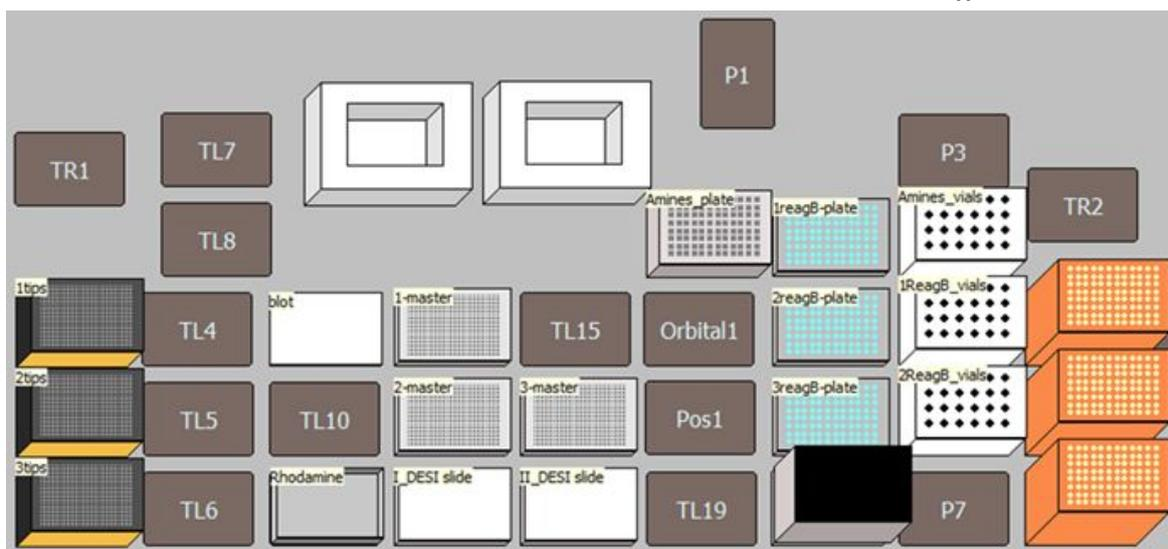
**Figure 7** (Top) Molecular structure of the 17 reagents used for the 3-by-8-hour experiment by group (amines, sulfonyl chlorides, acyl chlorides, and alkyl bromides). (Bottom) Deck layout of Biomek i7 during the case study. The different deck's estate can stage different types of equipment suitable for reagent preparation and DESI substrate pinning. A detailed description of the component of the deck is provided in the ESI (Table S.1).
