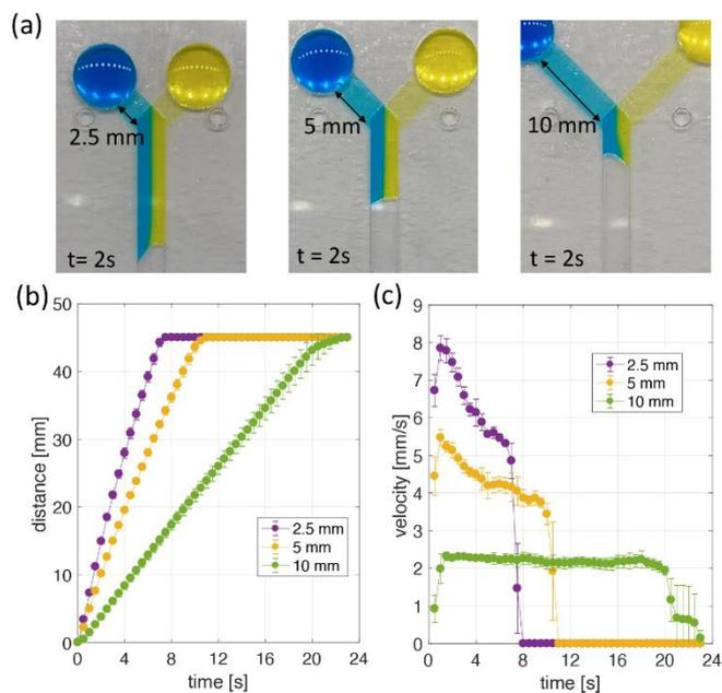
**Figure 5** (a) Y-shape devices with three different inlet length channels. All images show 2 s after blue and yellow dyes begin to flow through the main channel. (b) Flow distance in the main channel and (c) velocity variations over time for three different inlet channel devices. All data were calculated every 0.5 s and indicate the average (symbol) with the standard deviation (error bar) for three repeated experiments.
