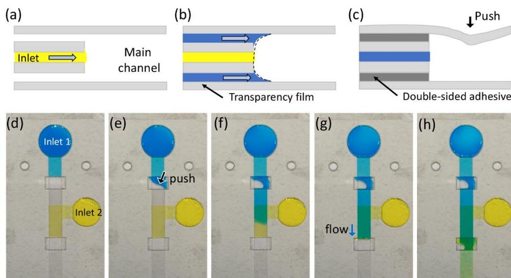
**Figure 3** Side-sectional schematics when (a) the flow stop, (b) burst valve system forming a single meniscus, and (c) push valve system. Sequential images of the valve device showing the moments of (d) flow stop, (e) push valve open, (f) push valve release, (g) form a single meniscus, and (h) burst valve release.
