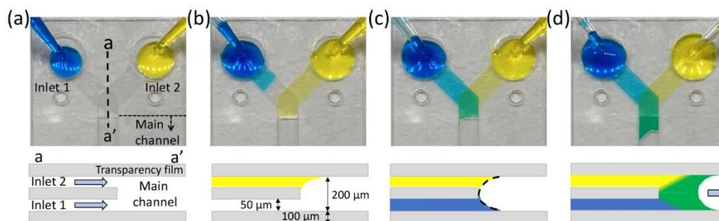
**Figure 2** Sequential images and side-sectional schematics of the simultaneous inflow system at the moments of (a) pipetting the solutions, (b) arriving the junction, (c) making a combined meniscus, and (d) entering into the main channel.
