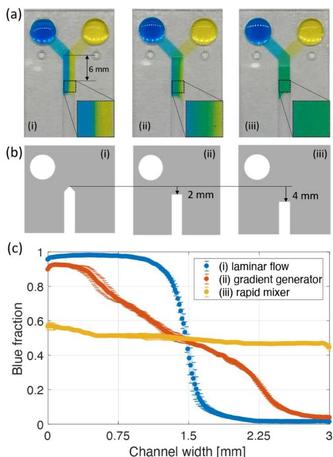
**Figure 4** (a) Three types of the Y-shaped device generating (i) non-mixing, (ii) a concentration gradient, (iii) fully mixing concentration profile. (b) Different geometries of the middle transparency layers. (c) Blue fraction distributions with respect to the channel width. Each value indicated in the plot calculated by averaging an enlarged image shown in Figure 4a. Error bars represent the standard deviation between experiments for each value.
