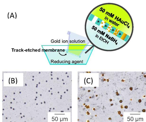
Figure 2. (A) Schematic of cBPE array fabrication using electroless plating method with gold. Optical microscope image of the surface of the track-etched membrane (B) before and (C) after electroless plating of gold.
