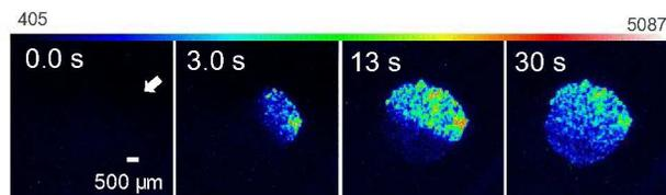
Figure 3. Time-lapse images of the high spatio-temporal resolution ECL signal of  $[\text{Fe}(\text{CN})_6]^{3-}$  solution spreading on the cBPE array in the sample chamber. Gain 255, exposure time 100 ms.
