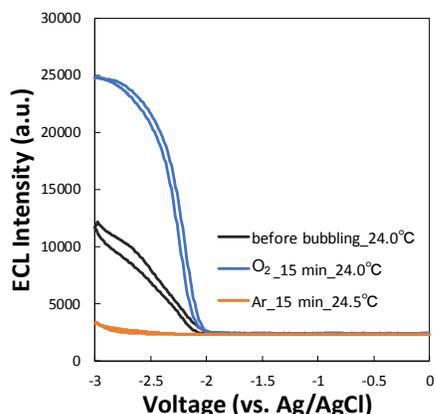
Figure 4. ECL intensities measured while sweeping the driving voltage on WE. (Black) PBS without gas bubbling, (blue) after O<sub>2</sub> gas bubbling for 15 min, and (red) after Ar gas bubbling for 15 min.
