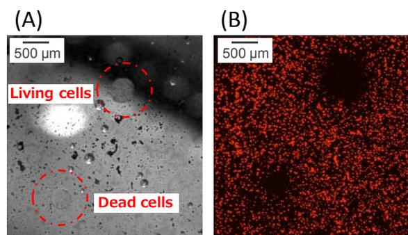
Figure 5. (A) Position of the spheroid recorded from below the detecting chamber with the CCD camera. (B) ECL image obtained by applying -2.6 V on WE with live/dead cells on the cBPE array surface.
