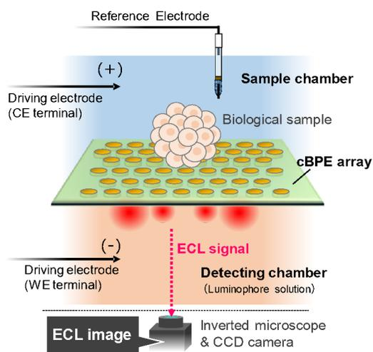
Figure 1. Schematic illustration of BEM.
