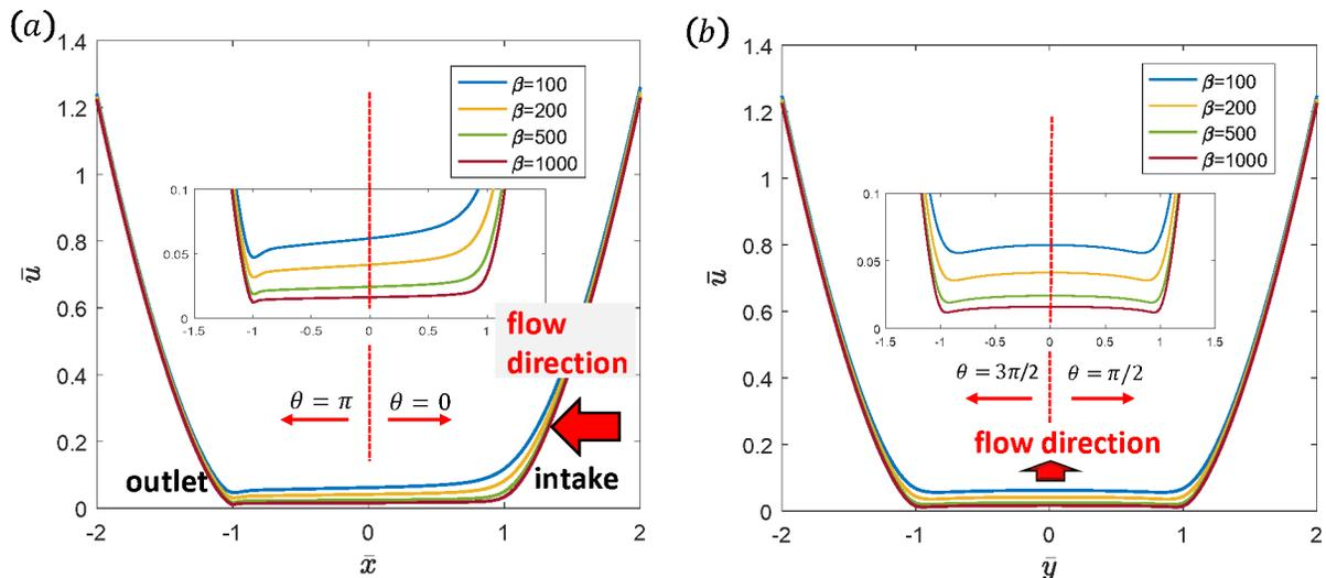
**Fig. 8** Film thickness profile at different cross-section; (a) cross-section along  $\bar{x}$  axis; (b) cross-section along  $\bar{y}$  axis. The results of different  $\beta = 100, 200, 500, 1000$  are presented. The imbedded figures show details of the film thickness at the ‘Hertz’ contact region.
