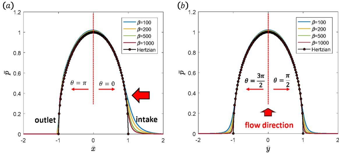
**Fig. 5** Hydrodynamic Pressure profile at different cross-section; (a) cross-section along  $\bar{x}$  axis; (b) cross-section along  $\bar{y}$  axis. The results of different  $\beta$  value are presented,  $\beta = 100, 200, 500, 1000$ . The Hertzian solution is plotted as comparison.
