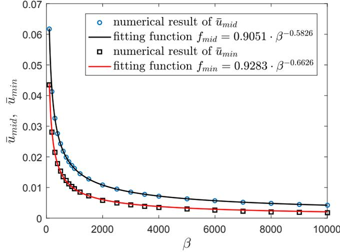
**Fig. 10** Dependence of liquid film thickness at  $\bar{r} = 0$  ( $\bar{u}_{mid}$ ) and minimum film thickness ( $\bar{u}_{min}$ ) on  $\beta$  . Fitting functions for  $\bar{u}_{mid}$  ,  $\bar{u}_{min}$  are also plotted.
