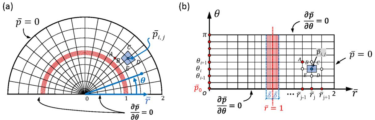
**Fig. 2** (a) A schematic of the calculation domain and the mesh in cylindrical coordinate. Note mesh is much denser in the radial direction at  $\bar{r} = 1$ . (b) Mapping the semicircular calculation into a rectangular calculation domain, with the boundary condition being applied.
