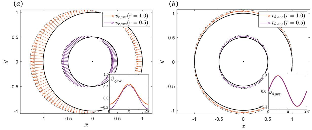
**Fig. 11** Components of the average velocity of the flow flowing into the two rings  $\bar{r} = 0.5$  and  $\bar{r} = 1.0$  (a) the averaged radial flow velocity  $\bar{v}_{r,ave}$ ; (b) the averaged swirl flow velocity  $\bar{v}_{\theta,ave}$ .
