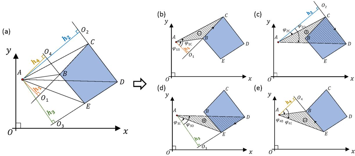
**Fig. 3** (a) Aim to calculate the deformation of the point,  $A$ , when it is subjected to a uniform pressure distribution on the quadrilateral  $BCDE$ ,  $AO_1 \perp BC$ ,  $AO_2 \perp CD$ ,  $AO_3 \perp DE$ ,  $AO_4 \perp EB$ . (b~e) Decomposition of a general quadrilateral into superposition of four triangles, the sign indicates addition or subtraction in the superposition process.
