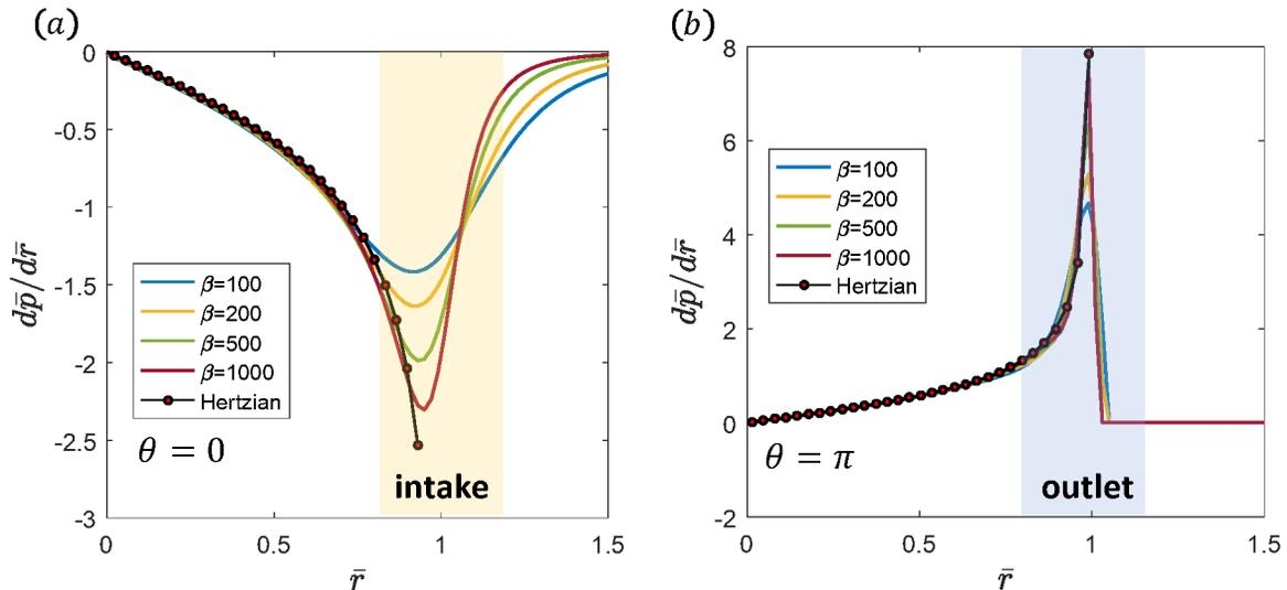
**Fig. 6** Pressure gradient in (a) the intake region ( $\theta = 0$ ) and (b) the outlet region ( $\theta = \pi$ ). The results of different  $\beta$  value are presented,  $\beta = 100, 200, 500, 1000$ . The Hertzian solution is plotted as comparison.
