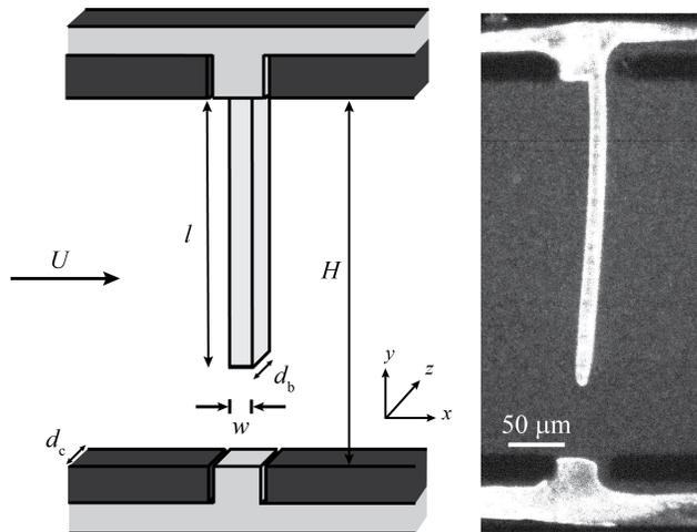
**Fig. 1** (a) Schematic of the cantilevered beam in the fabricated microchannel. The dark and light colored areas are composed of PDMS and photo-polymerized bounding wall and flexible beam respectively. (b) An image of the fabricated beam.
