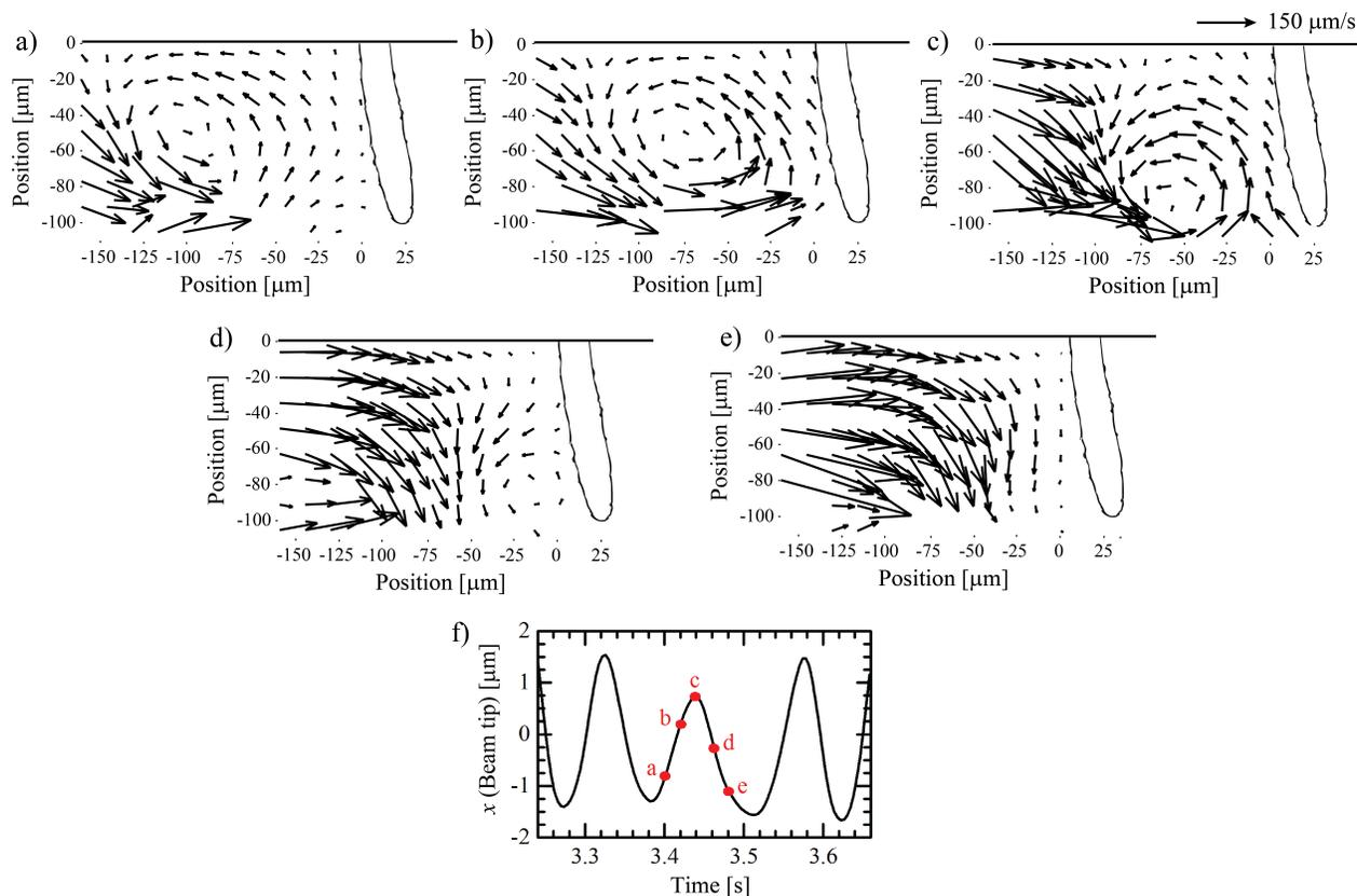
**Fig. 4** (a-e) PIV image sequence for flow past Beam 1 at  $Wi = 16$ . The time interval between each two consecutive images is 20 ms. The flow is from left to right. (f) The time history of the beam tip displacement with the solid dots (●) corresponding to the PIV image sequence from (a) to (e).
