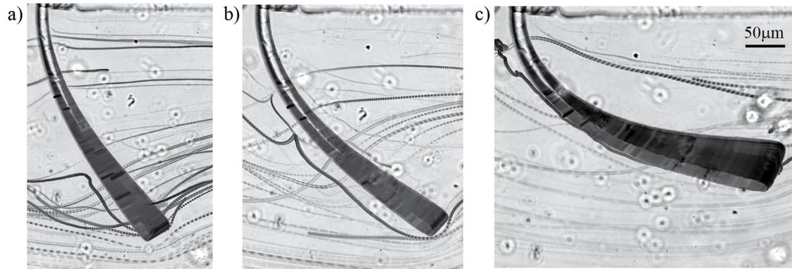
**Fig. 7** Bright field streakline image of viscoelastic flow past Beam 2 at varying Weissenberg numbers. (a)  $Wi = 5$ , (b)  $Wi = 8$  and (c)  $Wi = 12$ . The flow is from left to right.
