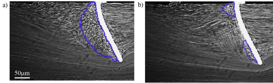
**Fig. 6** Dark field streakline image of flow fluctuations occurring in the upstream region of Beam 2 at  $Wi = 8$  for a time interval of 2.5 ms. The flow is from left to right.
