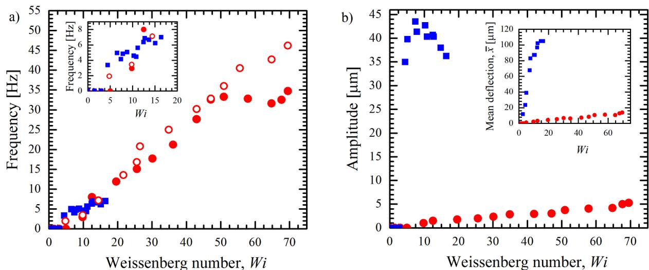
**Fig. 5** (a and inset) Frequency of Beam 1 (●) and Beam 2 (■) along with the frequency of fluctuating velocity vectors obtained from PIV images at a point  $2w = 34 \mu\text{m}$  upstream of the tip of Beam 1 (○) versus Weissenberg number. (b) Amplitude of Beam 1 (●) and Beam 2 (■) tip oscillations versus Weissenberg number. The inset is a plot of the mean deflection ( $\bar{x}$ ) observed during oscillations versus Weissenberg number.
