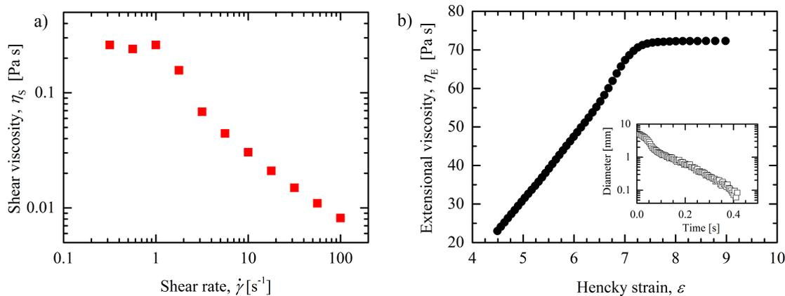
**Fig. 2** (a) Shear viscosity as a function of the shear rate and (b) extensional viscosity versus Hencky strain of the viscoelastic polymer solution. The inset is a representative plot of the diameter decay versus time recorded in a CaBER experiment.
