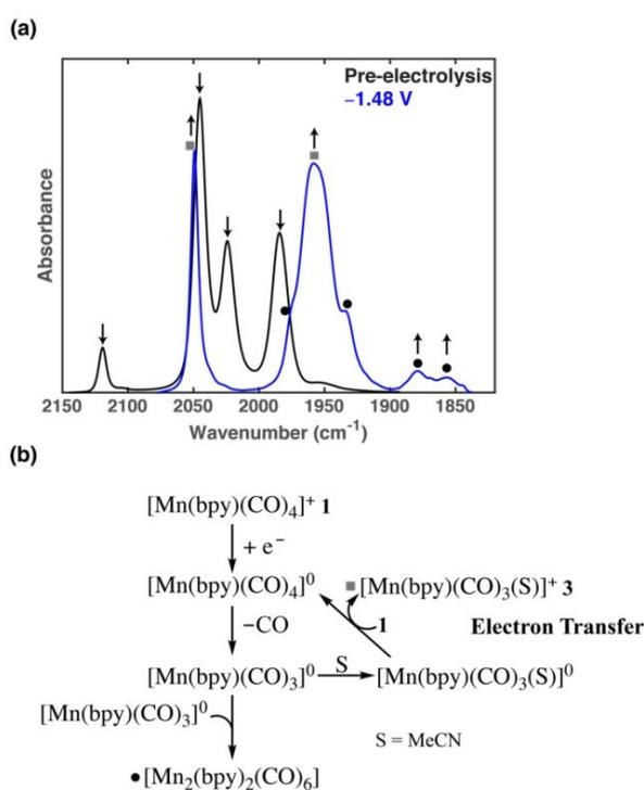
**Figure 8.** (a) IR spectral changes of **1** before and after a 5 minute bulk electrolysis at  $-1.48$  V vs.  $Fc/Fc^+$  under Ar. The new peaks correspond to the formation of two species: complex **3** (■) and the Mn-Mn bonded dimer (●). Schematic electrochemical reaction mechanism of **1** at the first reduction potential.
