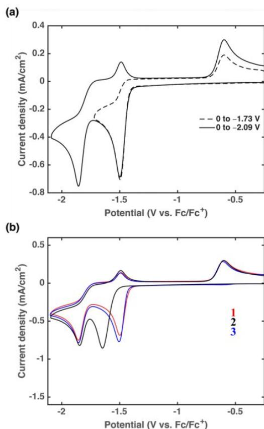
**Figure 4.** (a) CV data of **1** (1 mM) at two different switching potentials. The data were recorded at 250 mV/s under Ar in 0.1 M TBAH in MeCN with a 3-mm-diameter glassy carbon working electrode, a platinum foil counter electrode, and a Ag/Ag<sup>+</sup> nonaqueous reference electrode. All the potentials are referenced to Fc/Fc<sup>+</sup>. (b) CV data comparison for the three complexes under study. The other conditions were similar to those shown in panel a.
