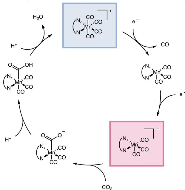
**Figure 1.** Proposed mechanism for  $\text{CO}_2$  reduction to  $\text{CO}$  by  $[\text{Mn}(\text{bpy})(\text{CO})_4]^+$  (blue box) by way of the active species  $[\text{Mn}(\text{bpy})(\text{CO})_3]^-$  (red box) in the presence of weak Brønsted acids.
