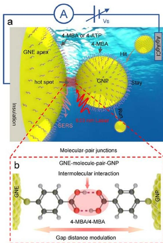
**Scheme 1** (a) Experimental setup and the “hit-stay-run” collision events of 40 nm diameter GNP on the apex of a partially insulated GNE by high-density polyethylene (HDPE). The radius of the GNE apex is in the range of 100-200 nm. (b) The structure of collision formed molecule-pair junction GNE-4-MBA/4-MBA-GNP junction. The size is not to scale.
