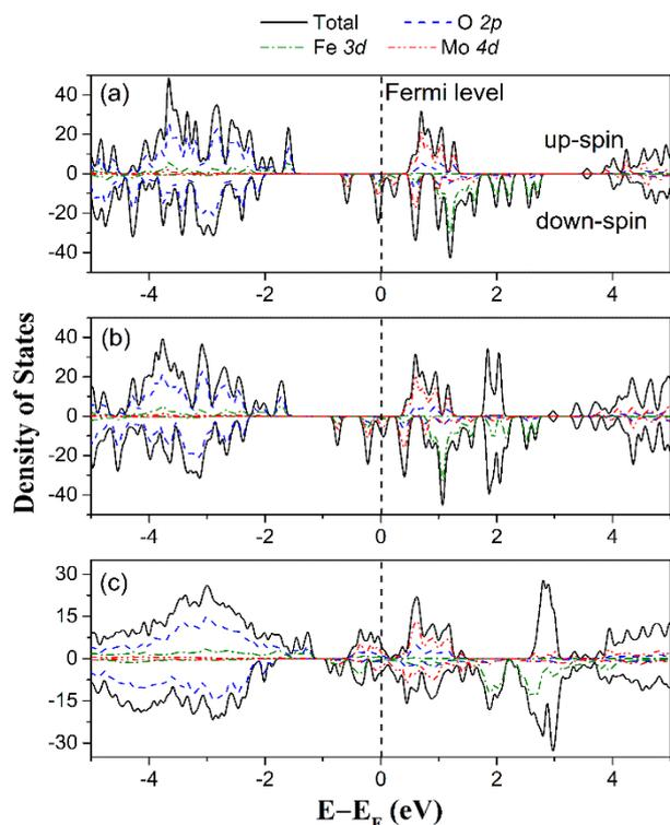
**Fig. 5** Total and partial density of states of (a) perfect  $\text{Sr}_8\text{Fe}_4\text{Mo}_4\text{O}_{24}$ ; (b) perfect  $\text{Sr}_7\text{LaFe}_4\text{Mo}_4\text{O}_{24}$ ; (c)  $\text{Sr}_7\text{LaFe}_4\text{Mo}_4\text{O}_{24}$  with 25% AD in the  $ab$  plane and a  $\text{O}^*$  along the  $\text{Fe}-\text{O}^*-\text{Fe}_{\text{Mo}}$ .
