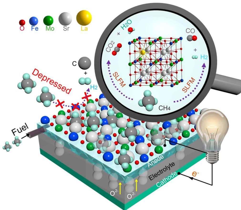
Electron doping-induced structure modification of double-perovskite anode material with enhanced electrocatalytic activities for methane oxidation in solid oxide fuel cells.
