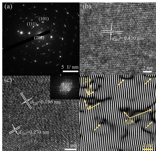
**Fig. 3** (a) SAED patterns of the  $\text{Sr}_{1.8}\text{La}_{0.2}\text{FeMoO}_{6-\delta}$  catalyst; (b, c) HRTEM image of the  $\text{Sr}_{1.8}\text{La}_{0.2}\text{FeMoO}_{6-\delta}$  catalyst. Inset is the corresponding FFT image; (d) Inverse FFT image of (c) with many anti-site defects marked with arrows.
