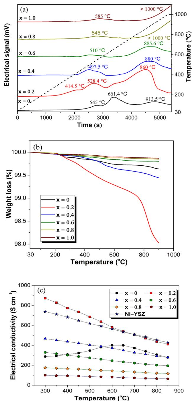
**Fig. 4** (a)  $\text{H}_2$ -TPR plots of  $\text{Sr}_{2-x}\text{La}_x\text{FeMoO}_{6-\delta}$  ( $0 \leq x \leq 1$ ) catalysts; (b) TGA profiles of  $\text{Sr}_{2-x}\text{La}_x\text{FeMoO}_{6-\delta}$  measured in  $\text{N}_2$ ; (c) Electrical conductivity of  $\text{Sr}_{2-x}\text{La}_x\text{FeMoO}_{6-\delta}$  and Ni-YSZ in  $\text{H}_2$ .
