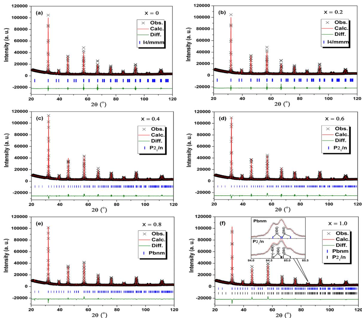
**Fig. 1** Rietveld refinement profiles of  $\text{Sr}_{2-x}\text{La}_x\text{FeMoO}_{6-\delta}$  to powder XRD collected at room temperature: (a)  $x = 0$  ( $I4/mmm$ ); (b)  $x = 0.2$  ( $I4/mmm$ ); (c)  $x = 0.4$  ( $P2_1/n$ ); (d)  $x = 0.6$  ( $P2_1/n$ ); (e)  $x = 0.8$  ( $Pbnm$ ); and (f)  $x = 1.0$  ( $Pbnm$ ). The inset in (f) shows the refinement profiles in comparison with  $P2_1/n$ .
