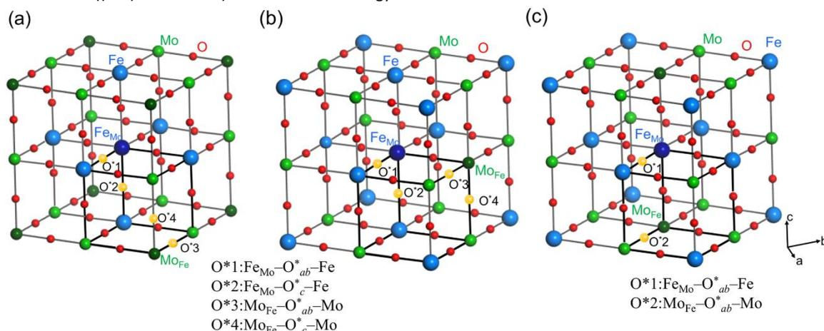
**Fig. 7** (a) Oxygen vacancies in Sr<sub>7</sub>LaFe<sub>4</sub>Mo<sub>4</sub>O<sub>24</sub> (4Sr<sub>1.8</sub>La<sub>0.2</sub>FeMoO<sub>6-δ</sub>) with anti-site defects: (a) along the diagonal, (b) in the *ab* plane, and (c) along the *c* axis of the cube.
