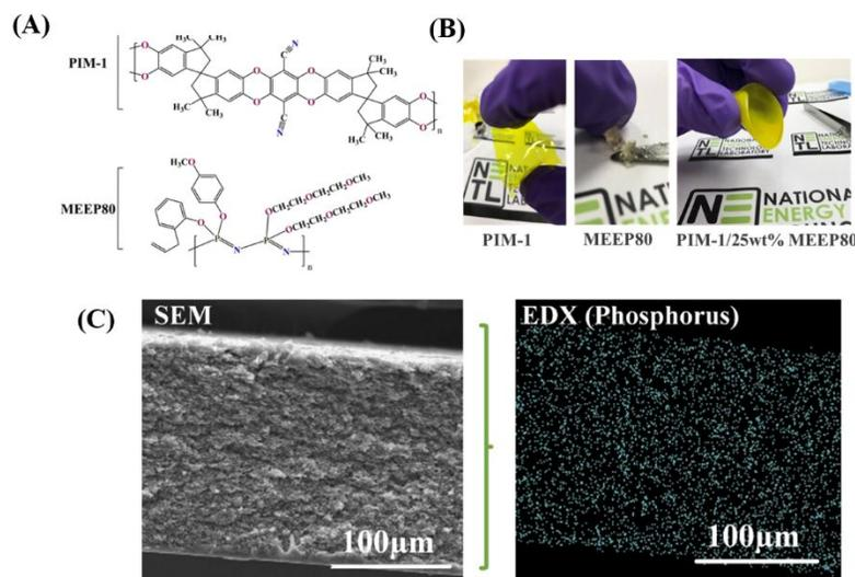
**Figure 1.** (A) Structures of PIM-1 and MEEP80, (B) photographs (left to right) of a brittle PIM-1 film, gel-like MEEP80 and a flexible PIM-1/25wt % MEEP80 films. (C) SEM image and EDX mapping of phosphorous in PIM-1/25 wt% MEEP80 showing the relatively uniform distribution of MEEP80.
