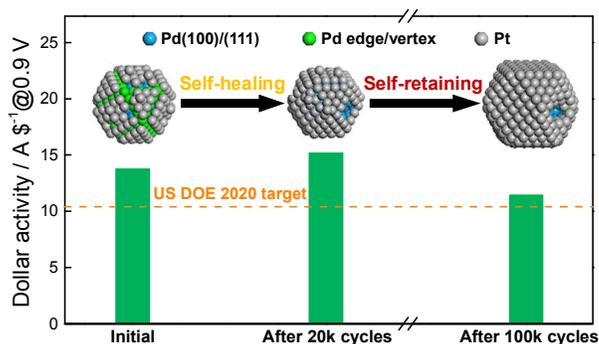
The structure-activity relationship of Pd-Pt<sub>ML</sub> core-shell electrocatalyst for the oxygen reduction reaction during up to 100k cycles of stability test is elucidated, and a new mechanism, the self-healing and self-retaining mechanism, is proposed to illuminate the ultra-high ORR stability of Pt<sub>ML</sub> electrocatalysts.
