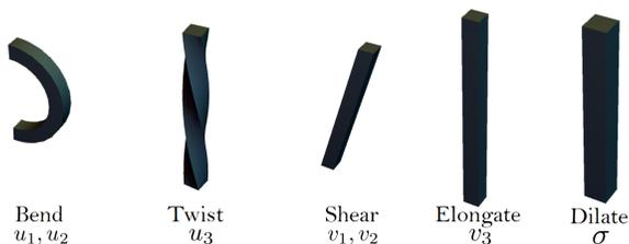
**Fig. 6** The fundamental deformations of a Cosserat rod with uniform parameters.
