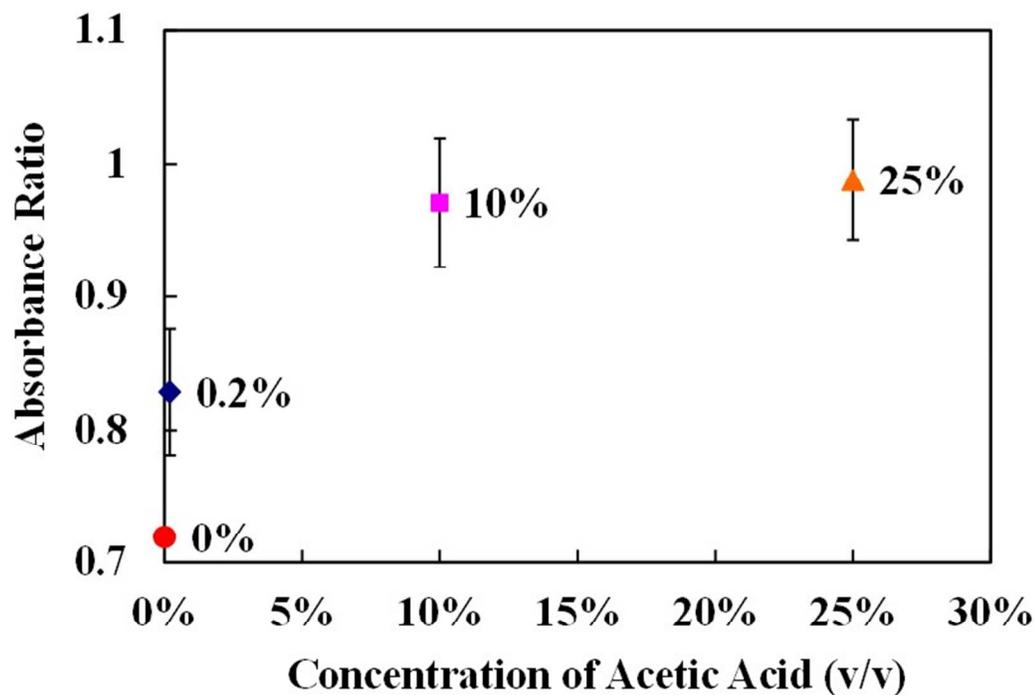
**Figure 7. Absorbance ratio of C=O stretching to -CH<sub>2</sub>- vibration in FTIR measurement (the experiments at each acid concentration were repeated at least 4 times).**
