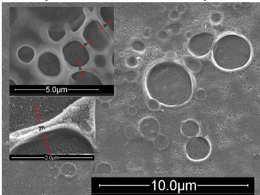
**Figure 6. SEM images of chitosan microcapsules used for measuring the thickness of the shell.**
