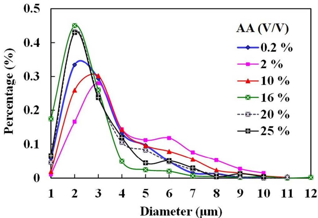
Figure 2. Size distributions of tetradecane with Nile red-filled cross linked chitosan microcapsules.
