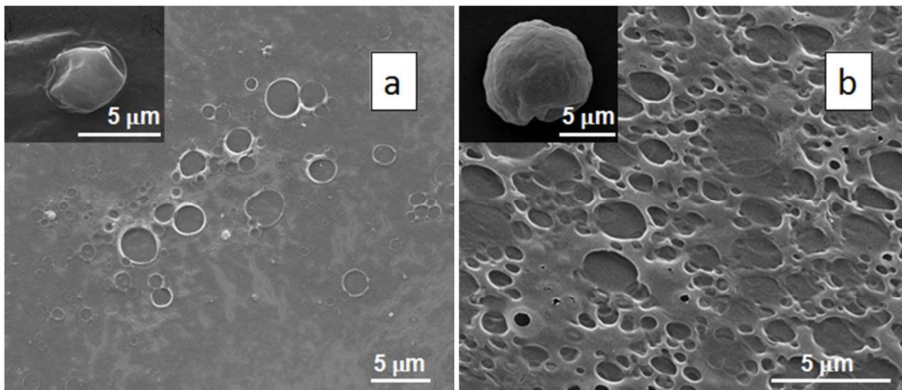
**Figure 5. SEM images of tetradecane-filled chitosan microcapsules (a. 0.2 %, b. 25 % at room temperature; inserts for heated microcapsules at 2% and 25%, respectively).**
