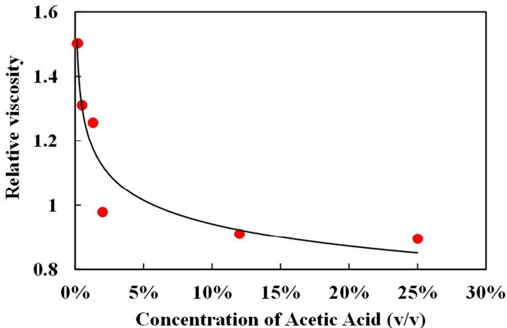
Figure 3. Relative viscosity of chitosan aqueous solutions with varying acetic acid concentrations, measured at  $22.3 \pm 0.2$  °C.
