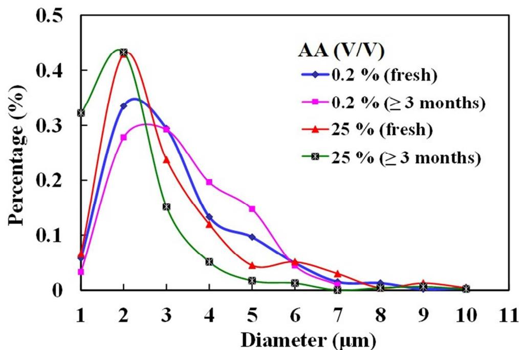
**Figure 4. Cross linked chitosan microcapsule size variation as a function of storage time and acetic acid concentration.**
