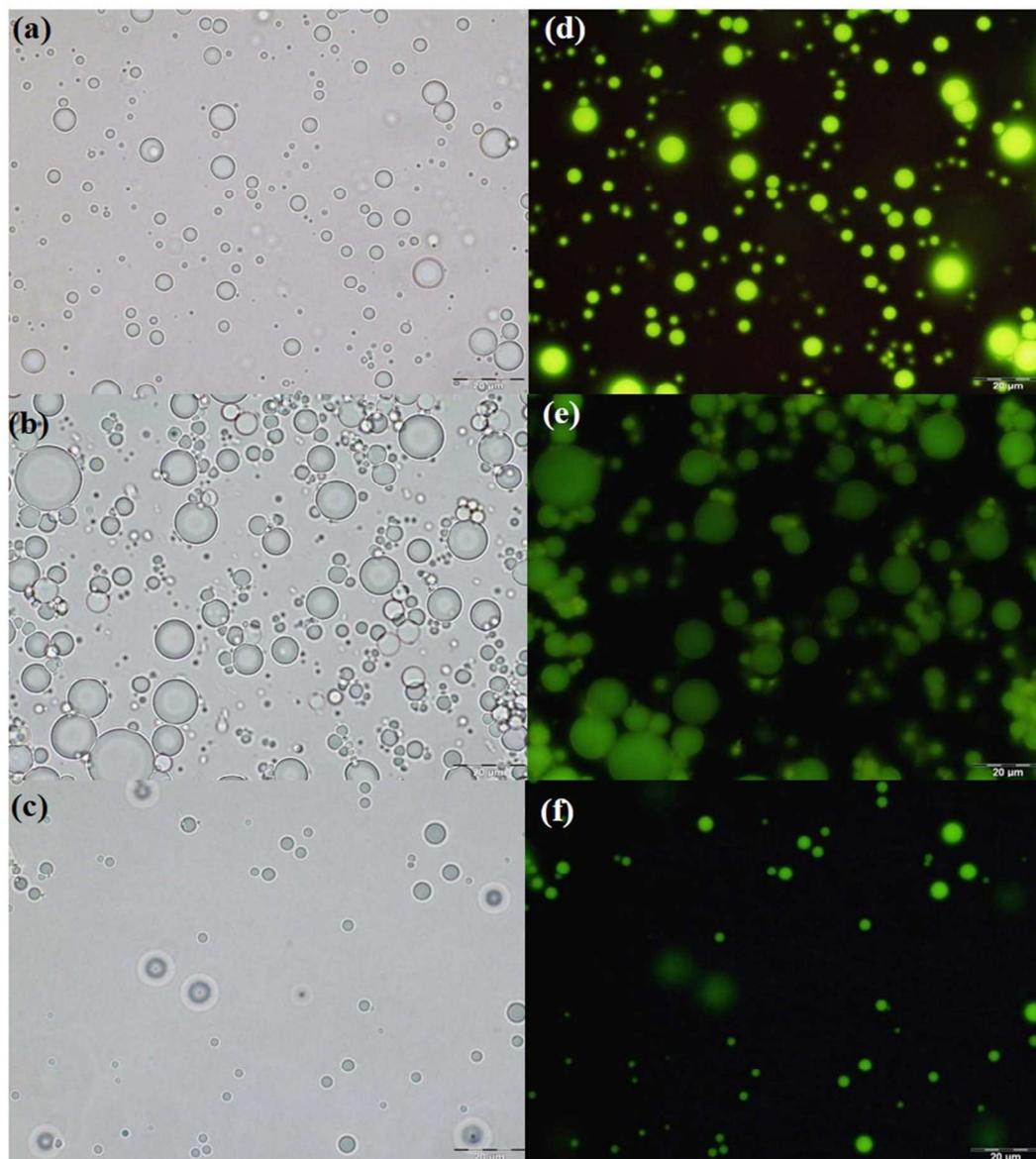
**Figure 1. Images of tetradecane (dyed with Nile red) filled chitosan microcapsules: Optical microscopy (OM) (a. 0.2 %, b. 2 %, c. 25 %) and fluorescence OM (d. 0.2 %, e. 2 %, f. 25 %). Scale: all images reported have a size of  $110 \mu\text{m} \times 147 \mu\text{m}$ .**
