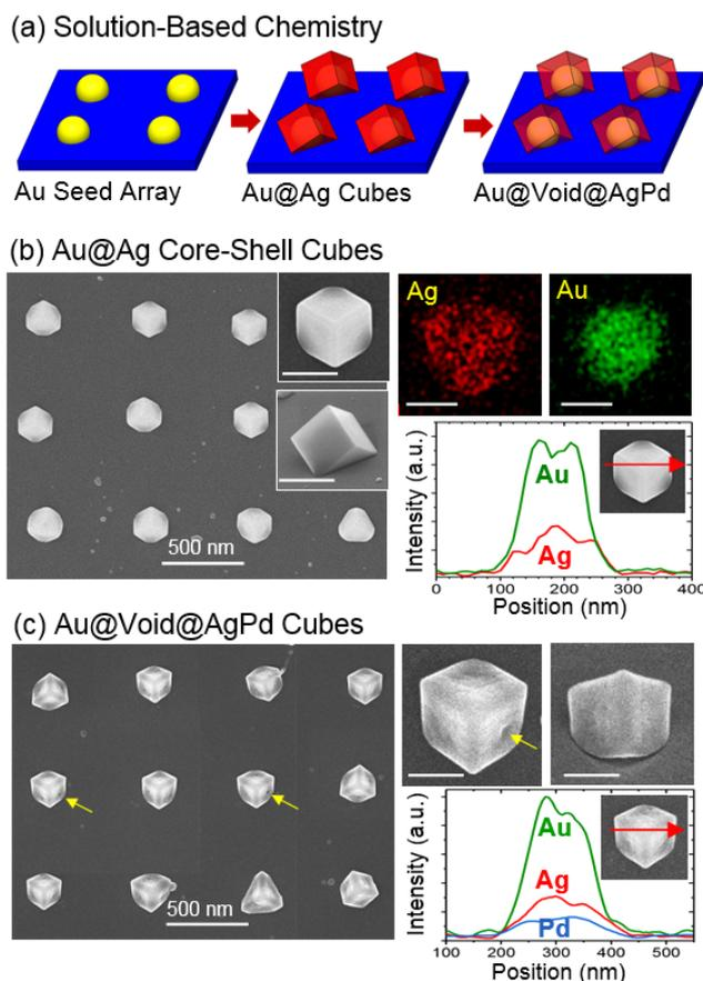
**Fig. 3** (a) Schematic showing the transformation that occurs as Au seeds are first transformed into an Au@Ag core-shell nanocube and then into an Au@void@AgPd core-void-shell structure using a two-stage solution-based synthesis. Top-view SEM images and the associated elemental maps and line scans for the (b) Au@Ag and (c) Au@void@AgPd structures (scale bar = 100 nm).
