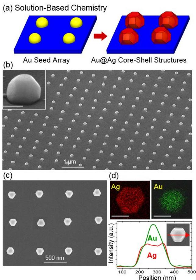
**Fig. 2** (a) Schematic showing the transformation that occurs when Au seeds are transformed into faceted Au@Ag core-shell structures using solution-based chemistry. SEM images of the Au@Ag structures taken from a (b) tilted- and (c) top-view. (d) EDS maps and line scans of an individual core-shell structure (scale bar = 100 nm).
