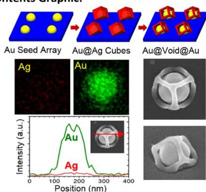
**Table of Contents Entry:** A nanofabrication strategy is presented for generating large-area arrays of metal nanostructures with an architectural complexity that rivals colloidal syntheses.
