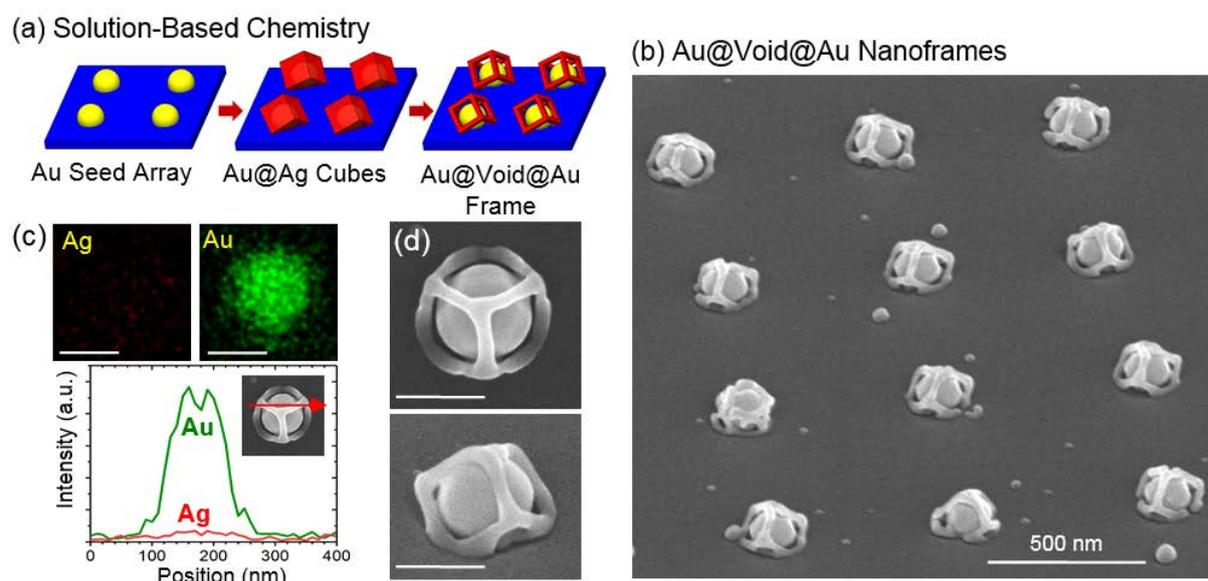
**Fig. 4** (a) Schematic showing the two stage synthesis that first transforms Au seeds into an Au@Ag core–shell nanocube and then into an Au@void@Au core–void–nanoframe. (b) Tilted-view SEM image of the framed structures formed in a periodic array. (c) Elemental maps and EDS line scans showing that nearly all of the Ag has been removed from the final structure and (d) top- and tilted-view high magnification images of a single structure (scale bar = 100 nm).
