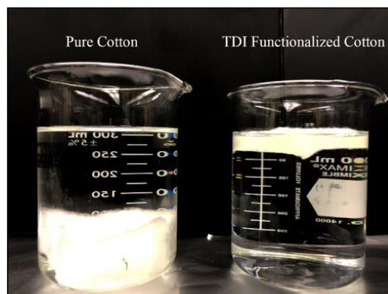
**Figure 2.** Difference of the hydrophilicity of the pure cotton and TDI functionalized cotton.
