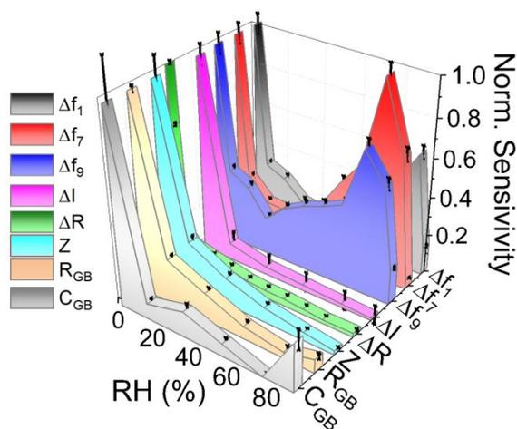
Figure 5. Normalized sensitivity of each sensing mode. Normalized sensitivity =  $S/S_{\max}$ , where  $S$  is sensitivity in units shown in (Fig. b), and  $S_{\max}$  is maximum sensitivity achieved for a given sensing mode.
