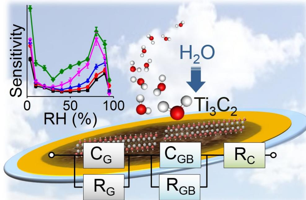
MXene ( $\text{Ti}_3\text{C}_2$ )-based humidity sensor demonstrates exceptional sensitivity to water vapor from 0.1%-95% RH with < 20 mTorr  $\text{H}_2\text{O}$  detection limit.
