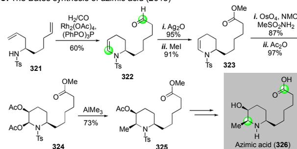
Fig. 55 Hydroformylation-aminal cyclization toward piperidine-containing natural products
