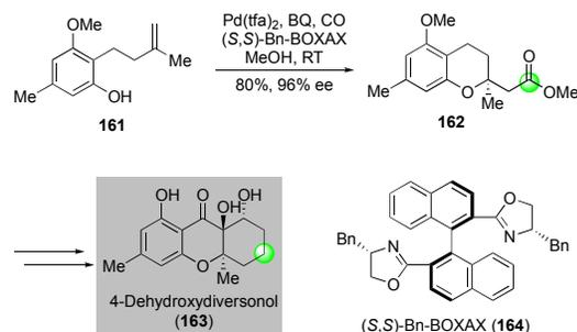
**Fig. 30** The Tietze synthesis of 4-dehydroxydiversonol (2008)
