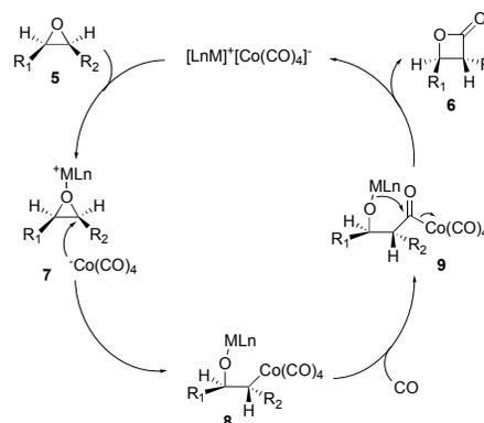
Fig. 3 Bimetallic [Lewis acid]<sup>+</sup>[Co(CO)<sub>4</sub>]<sup>-</sup>-catalyzed carbonylative  $\beta$ -lactone synthesis from epoxide
