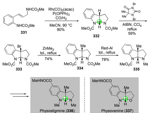
**Fig. 56** Hydroformylation-aminal cyclization toward pyrrolidine-containing natural products
