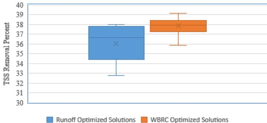
Figure 10. TSS removal percentage by the GIs for both WBRC-based and RV-based optimum solutions.
