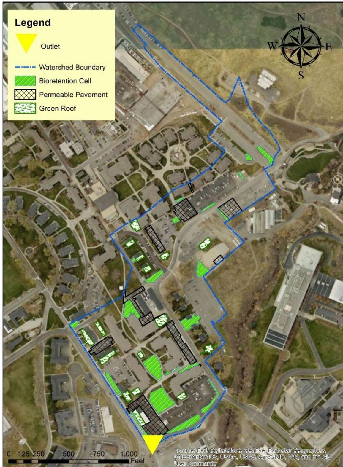
Figure 12. The configuration and distribution of GIs in the WBRC-optimum results.
