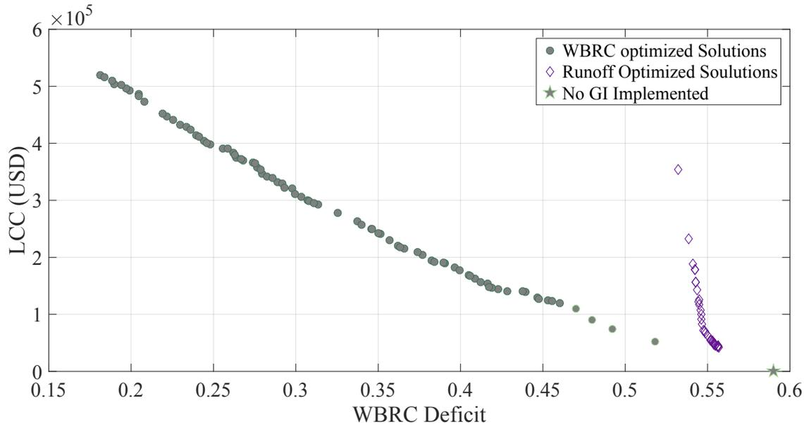
Figure 6. Pareto fronts on a WBRC Deficit versus LCC scale for both optimization sets.
