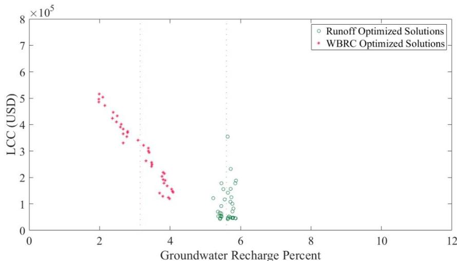
Figure 9. Ground Water Recharge percentage for both Pareto fronts (dashed lines show the average groundwater recharge values)
