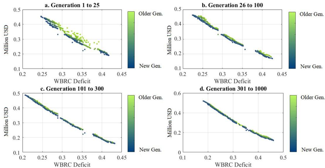
Figure 5. Shows the development of Pareto front **for the WBRC vs. LCC optimization set**. In all plots, lighter colors correspond to older generations, and dark blue ones are associated with new generations. Subfigure a) delineates generation 1 to 25; b) generations 26 to 100; c) major generations in 101 to 300; and d) major generations in 301 to 1000.
