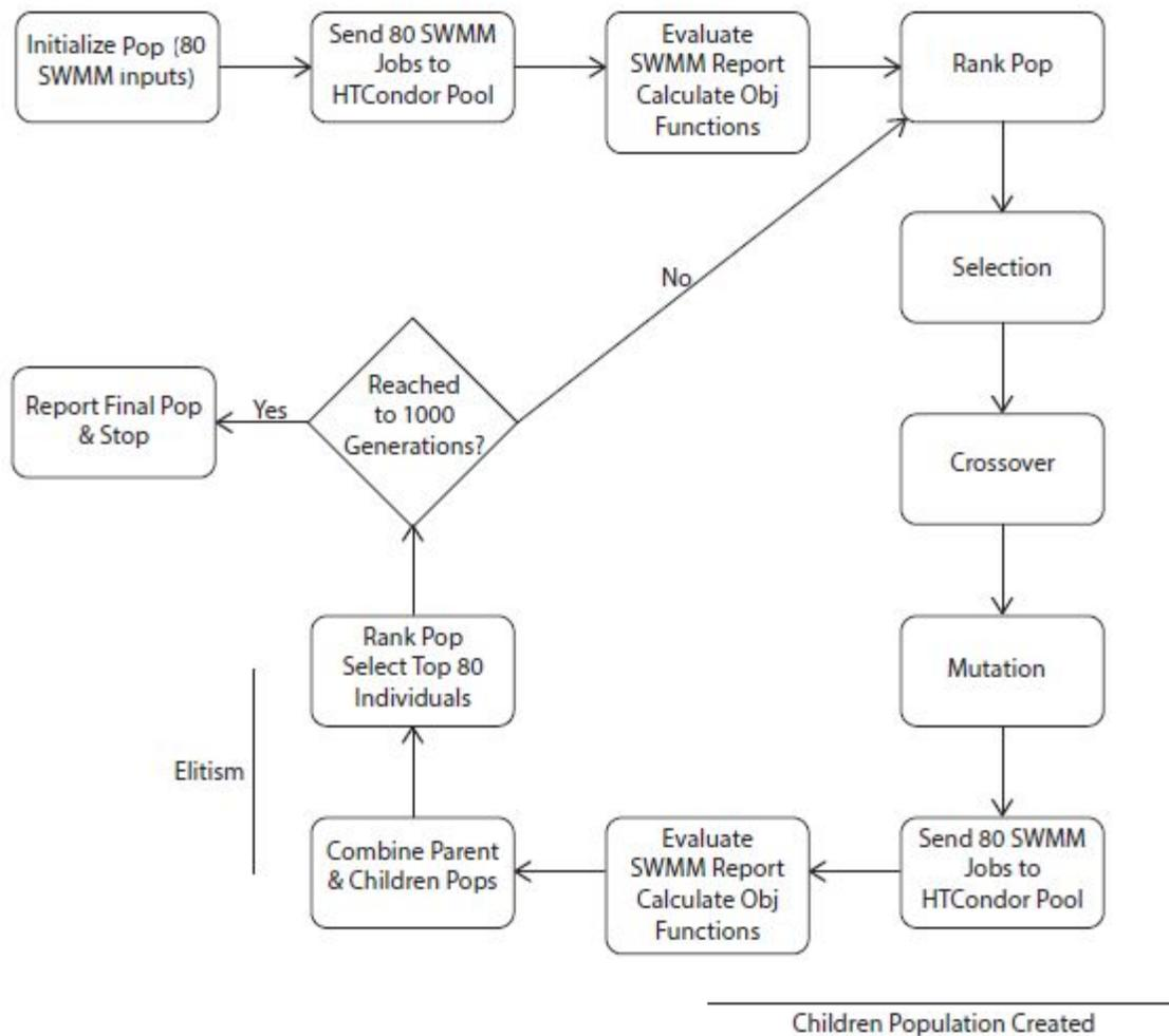
Figure 2. Flowchart showing the parallelized NSGA-II process. Note that Pop stands for the word “population”.
