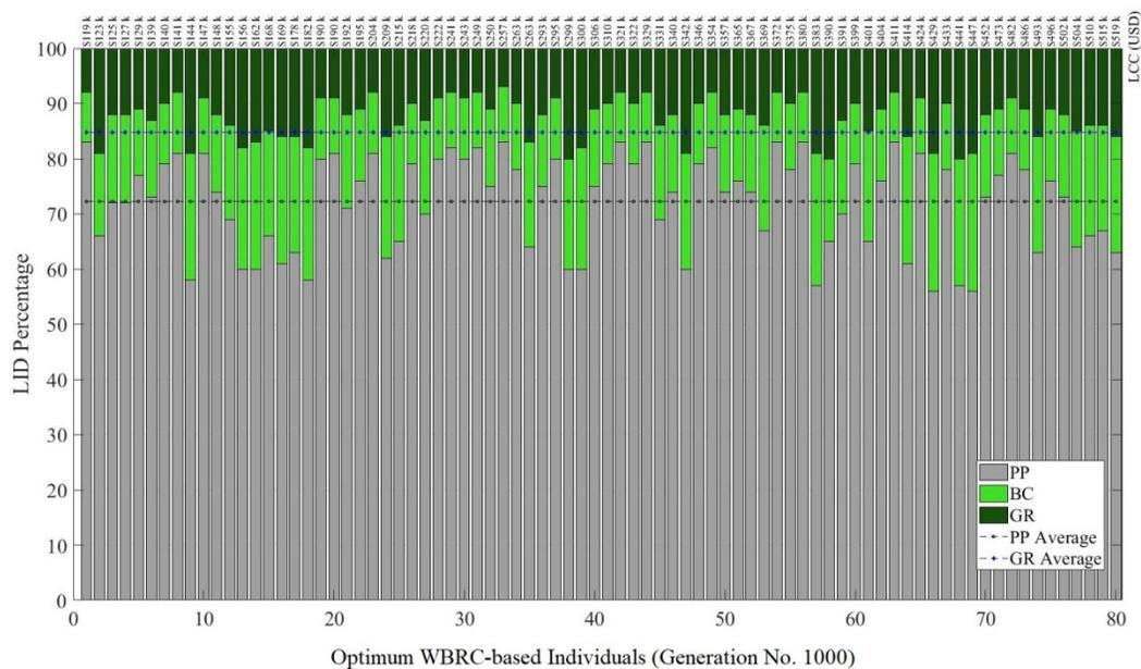
Figure 11. GI configuration of the optimum WBRC-based individuals. Each bar represents an optimum GI plan. Bars are sorted ascending based on LCC.
