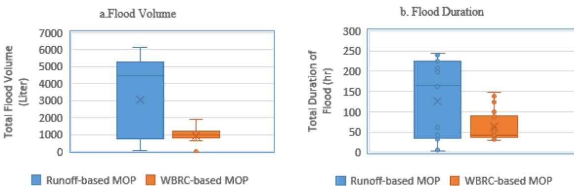
Figure 8. Flood protection analysis: a) the total **volume** of the flood for all flooded nodes for both Pareto fronts; and b) the total **duration** of the flood for all flooded nodes for both Pareto fronts.
