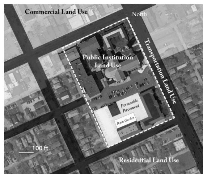
Figure 2. Holy Redeemer Church Site, Detroit, Michigan. This site includes a rain garden and a large area of permeable pavement for secondary parking.
