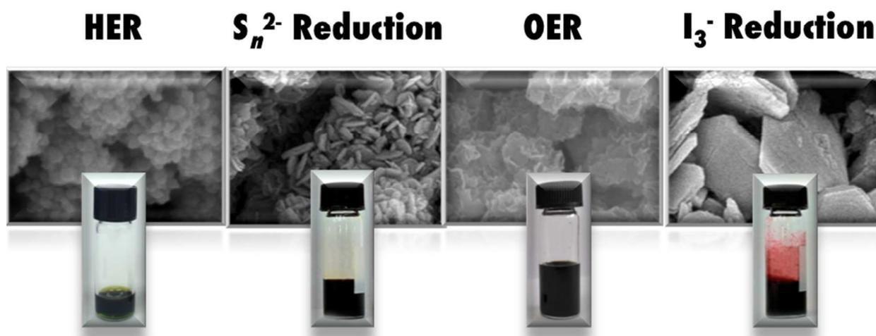
A thiol-amine solvent mixture was successfully utilized for the dissolution of bulk materials toward the solution deposition of chalcogenide electrocatalysts.
