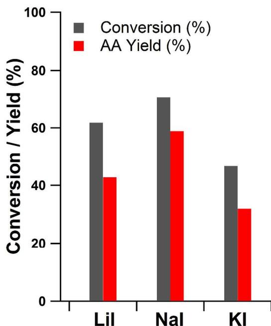
**Figure 1.** Effect of iodide sources on THFDCA conversion and AA yield. Conditions: 1 wt% THFDCA in 15 mL propionic acid using 0.1 M of each iodide salt, 1.8 g Nafion (0.1 M effective  $[H^+]$  based on IEC), and 500 psi  $H_2$  at 160 °C for 3 h.
