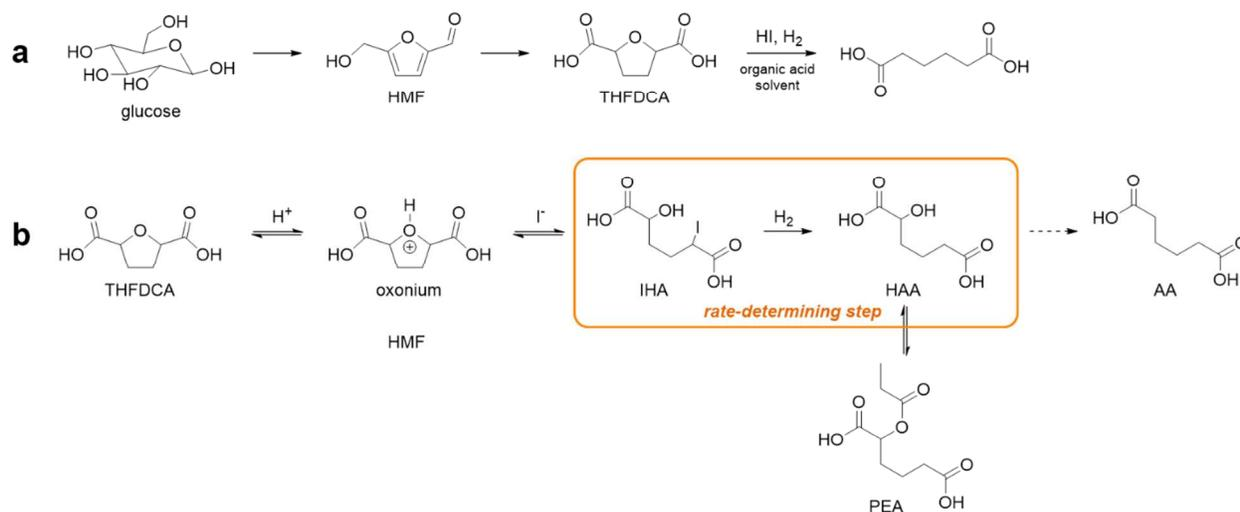
**Scheme 1.** AA formation from biomass-derived feedstocks from (a) glucose (dashed box emphasizes the ring-opening and hydrodeoxygenation steps without hydrogenation the COOH groups), and (b) tetrahydrofuran-2,5-dicarboxylic acid (THFDCA), illustrating the proposed reaction mechanism with C-I bond scission being the rate-determining step.<sup>5</sup> HMF = 5-hydroxymethylfurfural, THFDCA = tetrahydrofuran-2,5-dicarboxylic acid, IHA = 2-iodo-5-
