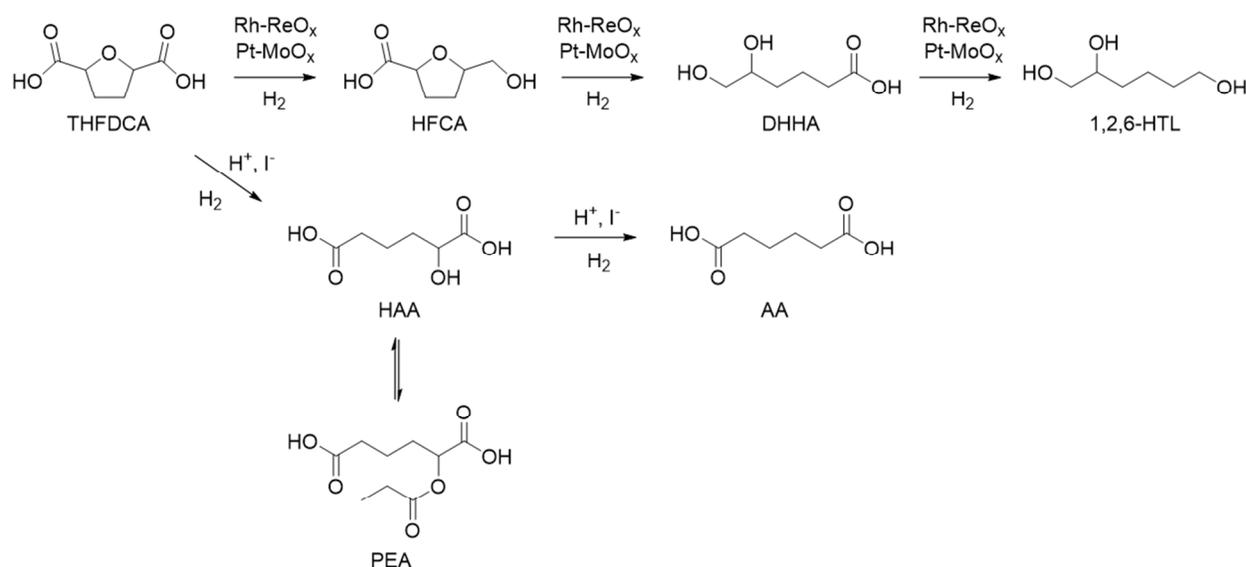
**Scheme 2.** Pathways from THFDCA demonstrating the preferential COOH hydrogenation over Rh-ReO<sub>x</sub> or Pt-MoO<sub>x</sub> catalysts and etheric C-O scission when iodide, molecular H<sub>2</sub>, and a proton source are used.
