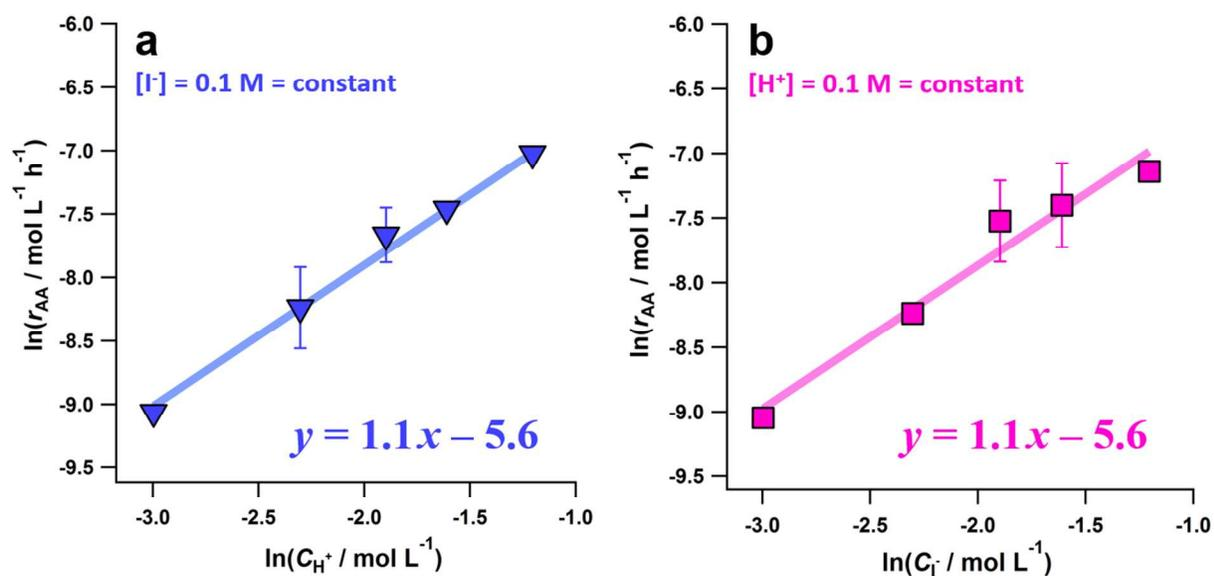
**Figure 2.** Reaction order with respect to (a) Nafion (proton concentrations based on IEC) at 0.1 M iodide concentration and (b) iodide at 0.1 M proton concentration (based on IEC of Nafion).
