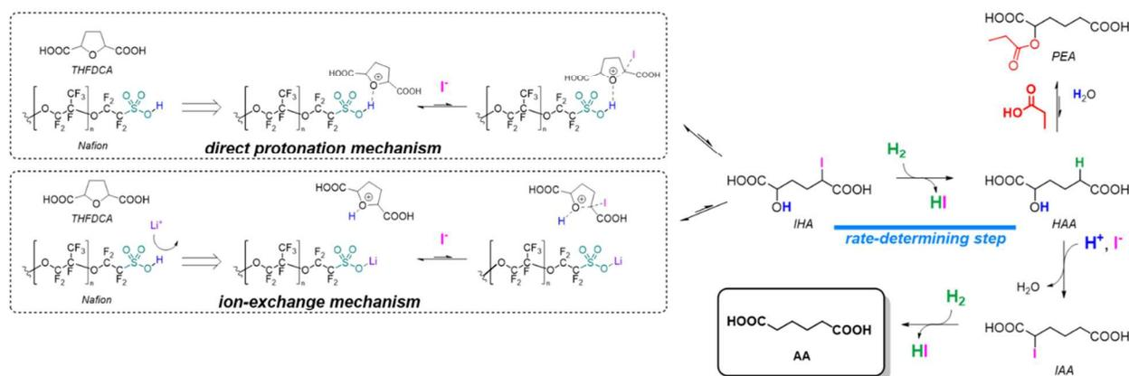
**Scheme 4.** Overall proposed mechanism for AA formation from THFDCA using solid acids and iodide sources suggesting (a) a direct protonation or (b) an ion-exchange mechanism.
