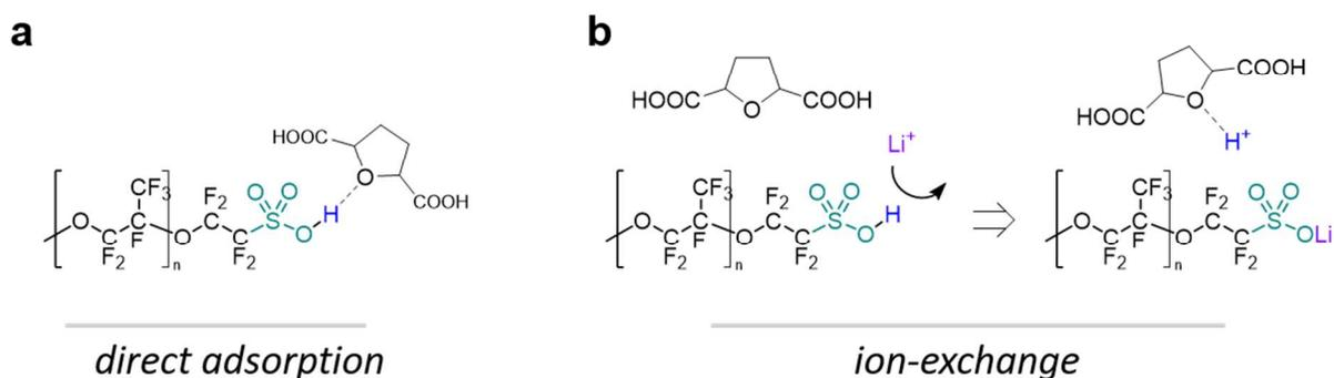
**Scheme 3.** Schematic distinguishing two possible mechanisms, including (a) direct adsorption of THFDCA to the active site on the solid acid material (heterogeneous chemistry), or (b) ion-exchange and solution-phase mediated protonation (homogeneous chemistry).
