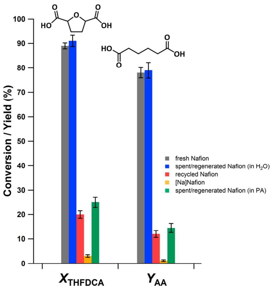
**Figure 3.** Comparison of fresh, spent, exchanged, and regenerated Nafion in THFDCA conversion and AA yield. Conditions: 1 wt% THFDCA in 15 mL propionic acid, 1.8 g Nafion (0.1 M H<sup>+</sup>), 0.3 M lithium iodide at 160 °C under 500 psi H<sub>2</sub> for reaction time of 4 h.
