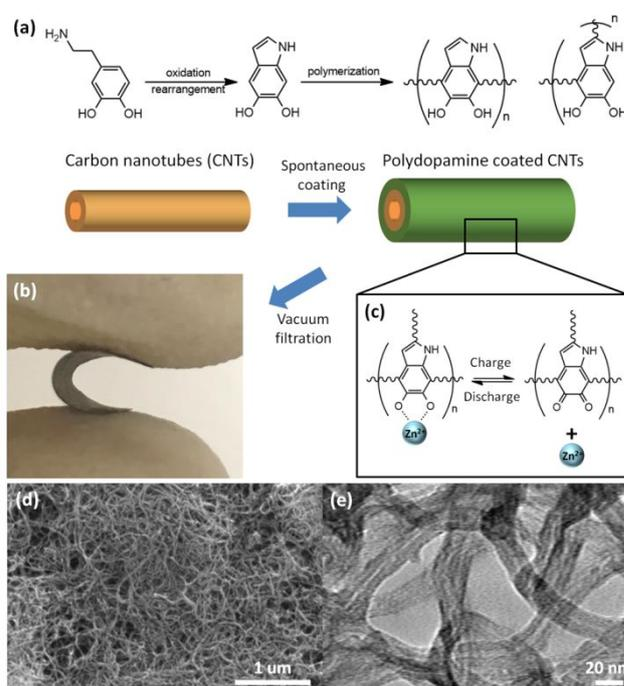
**Fig. 1** (a) Fabrication of PDA electrode by the spontaneous self-polymerization of dopamine on CNT supporting in basic aqueous solution. (b) Photo of a flexible free-standing CNT supported PDA thin film electrode. (c) Schematic of zinc ion adsorption by catechol and desorption by ortho-quinone when PDA at discharged or charged states, respectively. (d) Scanning electron microscopy (SEM) (e) Transmission electron microscopy (TEM) images of PDA electrode.
