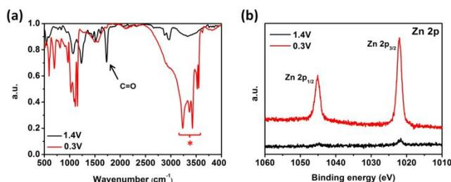
**Fig. 3** *Ex-situ* spectroscopic analysis of PDA electrodes at charged (1.4 V) and discharged (0.3 V) states. (a) FT-IR. (b) High resolution XPS Zn 2p. All electrodes were cycled between 0.3–1.4 V in 3.3 M ZnSO<sub>4</sub> aqueous electrolyte for 20 cycles at 200 mA/g, then charged or discharged to noted potentials. Peaks noted with the asterisk symbol represent N-H, O-Zn-O structure, and possible intermolecular bonds.
