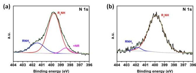
**Fig. 4** *Ex-situ* high resolution XPS N 1S spectrums of PDA electrodes. (a) Before cycling. (b) After cycling.
