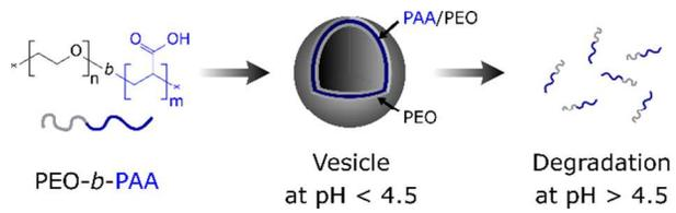
Double-hydrophilic diblock copolymers can assemble into pH-switchable containers for the encapsulation and release of cargo across biologically-relevant pH ranges.
