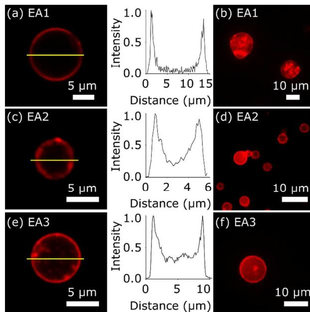
**Fig. 1** Formation of PEO-PAA vesicles. (a,c,e) Confocal micrographs, normalized intensity profiles, and (b,d,f) epifluorescence micrographs of EA1, EA2, EA3 vesicles at pH 2.3
