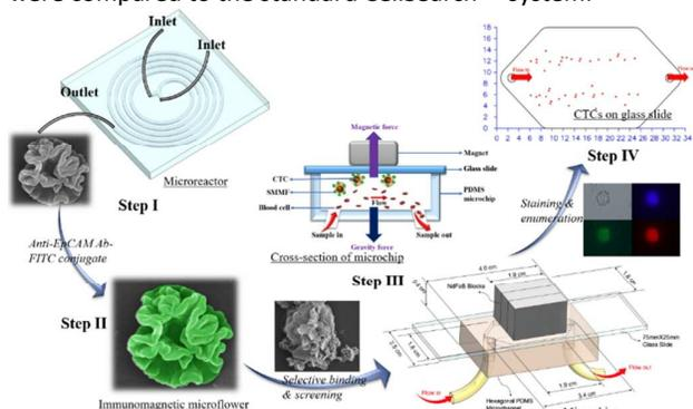
**Figure 1.** Schematic workflow showing the step-by-step process of microfluidics-enabled synthesis of SMMF toward CTCs screening.
