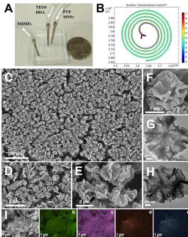
**Figure 2.** Microfluidic synthesis and characterization of SMMF. (A) The photograph showing the microfluidic device used in
