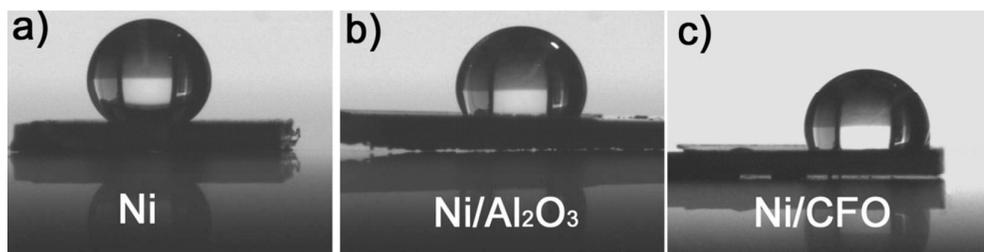
Fig. 8 Optical photographs of an aqueous sodium chloride droplet (7  $\mu\text{m}$ ) onto the surface of (a) Ni, (b) Ni/Al<sub>2</sub>O<sub>3</sub> and (c) Ni/Co<sub>2</sub>FeO<sub>4</sub> porous films.
