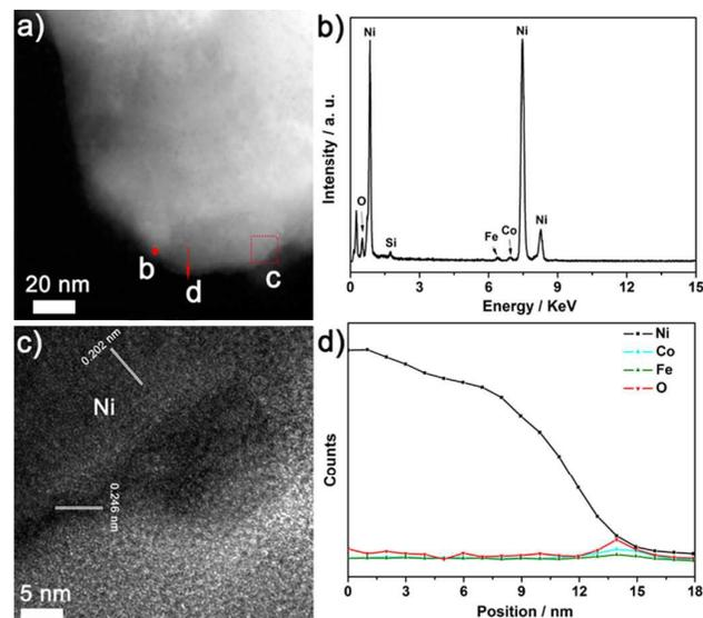
**Fig. 6** a) TEM image of the cross sectional view of Ni/Co<sub>2</sub>FeO<sub>4</sub> sample; b) EDX spectrum corresponding to the red dot "b" in a); c) HRTEM image of the area enclosed with the red square labeled as "c" in panel a); d) line-scan STEM-EDX analysis across the edge depicted with the red arrow "d" in panel a).
