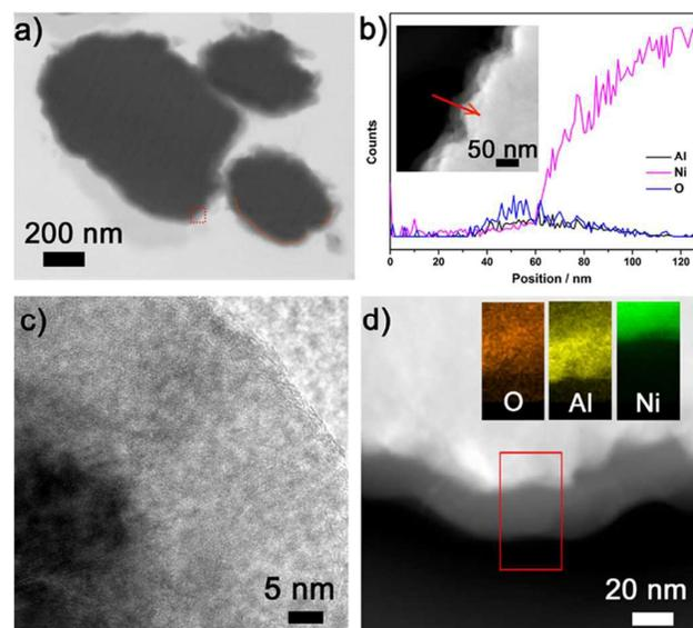
**Fig. 4** a) SEM image of A3 nanocomposite slice; b) line-scan STEM-EDX analysis across the interface between Ni and  $\text{Al}_2\text{O}_3$ , as indicated by the red arrow in the insert STEM image; c) HRTEM image of the area enclosed with the red dotted square in a); d) EDX elemental distribution of O, Al and Ni in the interfacial area enclosed within the red rectangle.
