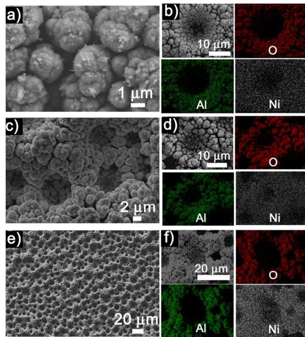
**Fig. 3** On-top SEM images of a) A1, c) A2 and e) A3 nanocomposites. EDX mapping distribution of Al, O, and Ni elements in b) A1, d) A2 and f) A3 composites, obtained from the zoomed SEM images shown on the left.
