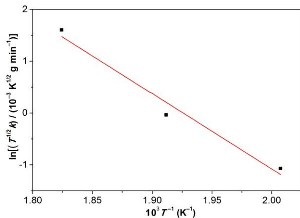
**Fig. 6** Temperature dependence of the mass loss for [Gdm-H][NfO] based on the IGA results shown in Fig. 5. Such a plot yields a slope of  $-\Delta_{\text{vap}}H/(1000R)$ , where  $\Delta_{\text{vap}}H$  is the enthalpy of vaporization,  $R$  is the universal gas constant, and  $k$  equals to  $dm/dt = m_0(da/dt)$ , which is the rate of mass loss per unit area shown in eqn. 3. Correlation of coefficient ( $R^2$ ): 0.95053.
