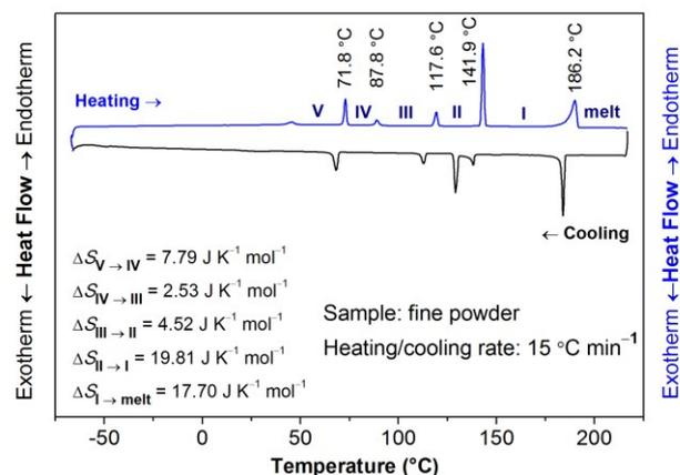
**Fig. 7** DSC thermograms of [Gdm-H][NfO] in the form of fine powders measured at  $15 \text{ °C min}^{-1}$  for both the heating and cooling scans. The onset 55 temperatures and entropy changes for each phase transition during the heating scan are given. Each solid phase is labeled by Roman numerals with the highest temperature solid phase denoted by phase I. The melt phase is also indicated. The peak temperature of melting is  $190 \text{ °C}$ .
