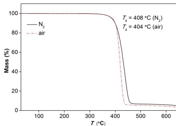
Fig. 4 TGA traces of [Gdm-H][NfO] in nitrogen gas and air, respectively. Heating rate: 5 °C min<sup>-1</sup>; gas flow rate: 50 mL min<sup>-1</sup>; mass of sample: 16.850 mg (nitrogen gas) and 16.630 mg (air).
