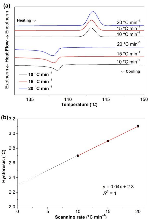
**Fig. 8** (a) DSC curves of [Gdm-H][NfO] at different heating/cooling rates showing in particular the phase transition of II → I during the heating scan and the reverse phase transition during the cooling scan; (b) The corresponding limiting temperature hysteresis (2.30 °C) estimated from the scans extrapolated to a scanning rate of 0 °C min<sup>-1</sup>, demonstrating a first-order solid-solid phase transition. Correlation of coefficient ( $R^2$ ): 1.
