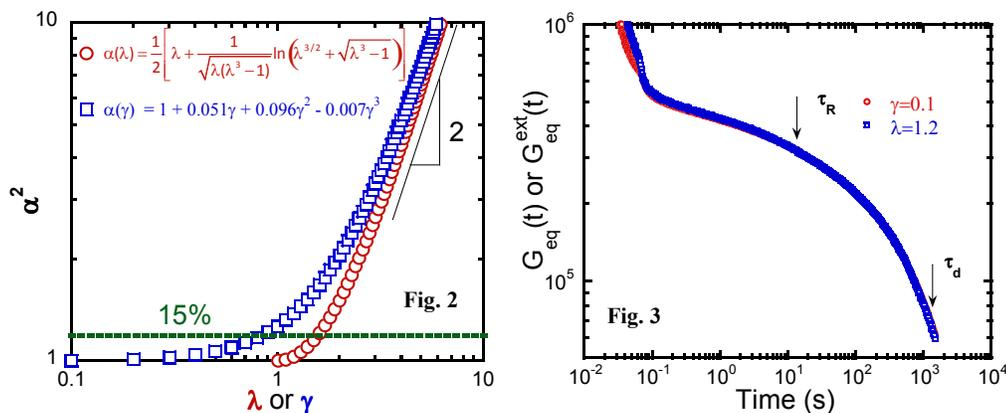
Figure 2 The chain stretching factor  $\alpha^2$  versus the imposed strain for either shear or extension according to tube model. The chain stretching would elevate the shear stress by 13 % for  $\gamma = 0.7$  and extensional stress by 15% for  $\lambda = 1.5$ .
