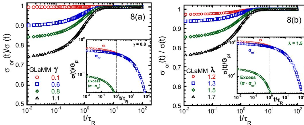
Figure 8 Orientational contribution  $\sigma_{or}$  to the total stress  $\sigma$  for both (a) shear and (b) extension calculated by the GLaMM model. Note that insets are the total stress  $\sigma$ , the orientational stress  $\sigma_{or}$ , and excess stress  $(\sigma - \sigma_{or})$  at  $\gamma = 0.8$  for shear and  $\lambda = 1.5$  for extension, respectively.
