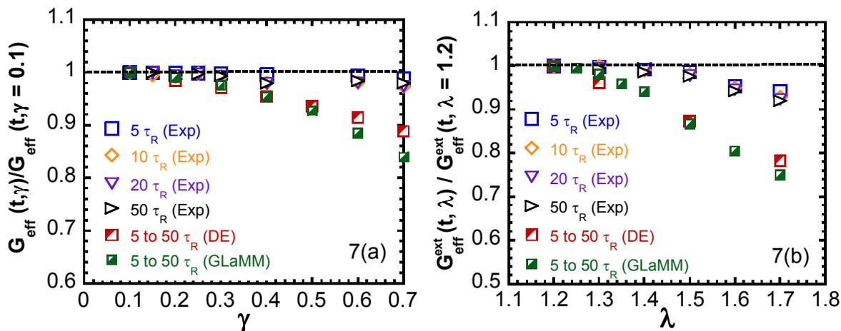
Figure 7 Normalized relaxation moduli based on experiment, the original Doi-Edwards tube model and the GLaMM model at "long time" from  $5 \tau_R$  to  $50 \tau_R$  for both (a) shear and (b) extension. The results from both the DE tube model calculation and the GLaMM model calculation are identical at different times from 5 to  $50 \tau_R$ .
