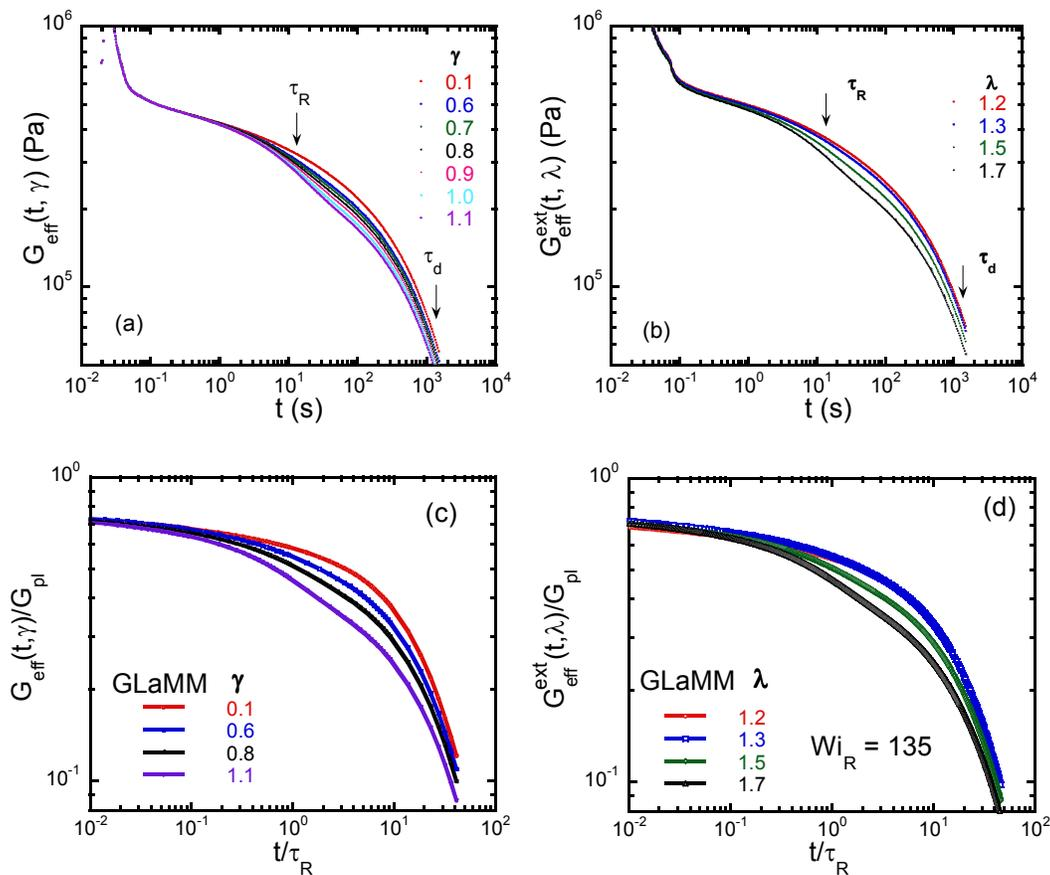
Figure 6 DE tube model calculation of shear modulus for a range of  $\gamma$  from 0.1 to 1.1 (a), and extensional relaxation modulus for stretching ratio  $\lambda$  ranging from 1.2 to 1.7 (b). The GLaMM model calculation of shear relaxation modulus for a range of  $\gamma$  from 0.1 to 1.1 (c), and extensional relaxation modulus for the stretching ratio  $\lambda$  ranging from 1.2 to 1.7 (d).
