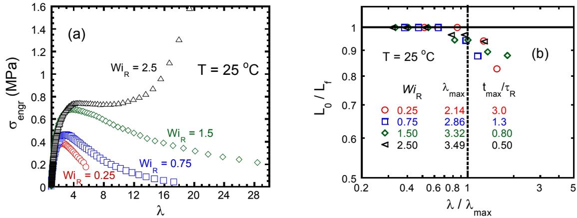
Figure 13 (a) Engineering stress  $\sigma_{\text{engr}}$  versus stretching ratio  $\lambda$  for startup extension at four values of  $Wi_R$  at  $25^\circ\text{C}$ . (b) The ratio of the initial specimen length  $L_0$  to the final recovered length after it has been stretched to the various elongation ratio both before and after the engineering stress maximum at  $\lambda_{\text{max}}$ , at four different Hencky rates of 0.01 to 0.1 at  $25^\circ\text{C}$  where the Rouse time is 25 s.
