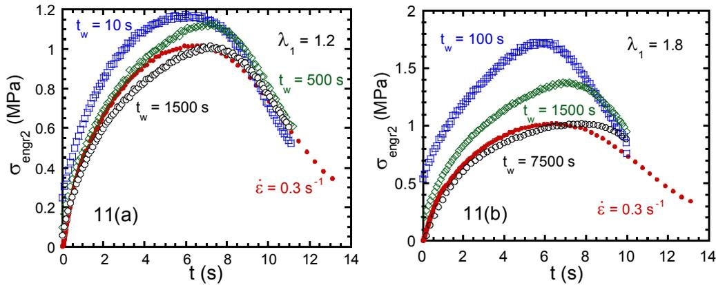
Figure 11 Engineering stress  $\sigma_{\text{engr2}}$  as a function of time, resulting from the startup extension applied at the various stages (designated by  $t_w$ ) during the stress relaxation from three different step extension of (a)  $\lambda_1 = 1.2$  and (b)  $\lambda_1 = 1.8$  respectively. The solid dots represent the stress vs. time curve from an equilibrium sample (i.e.,  $\lambda_1 = 0$ ) in terms of  $\sigma_{\text{engr}} = F/A_0$ .
