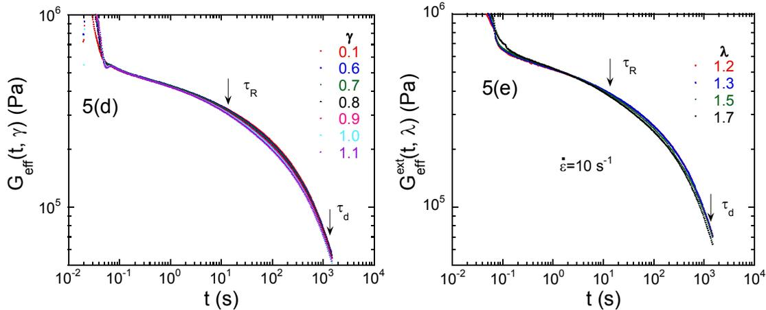
Figure 5 (a) Relaxation modulus as a function of time for different magnitudes of the step-wise shear, ranging from  $\gamma = 0.1$  to 1.1, imposed within 0.04~0.06 s. (b) Relaxation modulus as a function of time for different stretching ratio  $\lambda$  ranging from 1.2 to 1.7, imposed with a Hencky rate of  $10 \text{ s}^{-1}$ . (c) The amount of vertical shift due to strain softening. (d) and (e) replots of (a) and (b) after the vertical shifts according to (c).
