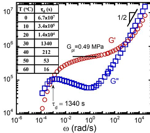
Figure 1 Small amplitude oscillatory shear measurements of SBR153K at 30 °C. The reptation time is  $\tau_d = 1340$  s. The inset shows the Williams-Landel-Ferry (WLF) shift for this sample for a temperature range from 0 °C to 60 °C.
