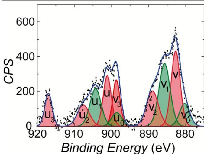
**Figure 4.** XPS Ce 3d core level spectrum of (011)CGO nanowires grown on (011)LAO substrates by RTA at 1000 °C, 20 °C s<sup>-1</sup> for 5 min in O<sub>2</sub> atmosphere. The fitted components in green and red correspond to Ce<sup>3+</sup> and Ce<sup>4+</sup> ions, respectively.
