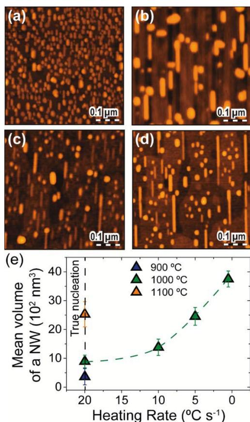
**Figure 7.** AFM images of nanowires grown on (011)LAO substrates in O<sub>2</sub> without dwell time at: (a) 1000 °C, 20 °C s<sup>-1</sup>, (b) 1100 °C, 20 °C s<sup>-1</sup>, (c) 1000 °C, 5 °C s<sup>-1</sup> and (d) 1000 °C, 0.5 °C s<sup>-1</sup>. (e) Dependence of the mean volume of a NW with the heating rate and temperature, extracted from AFM images (a-d). The black dashed vertical line indicates the heating rate where the contribution of coarsening is considered to be negligible.
