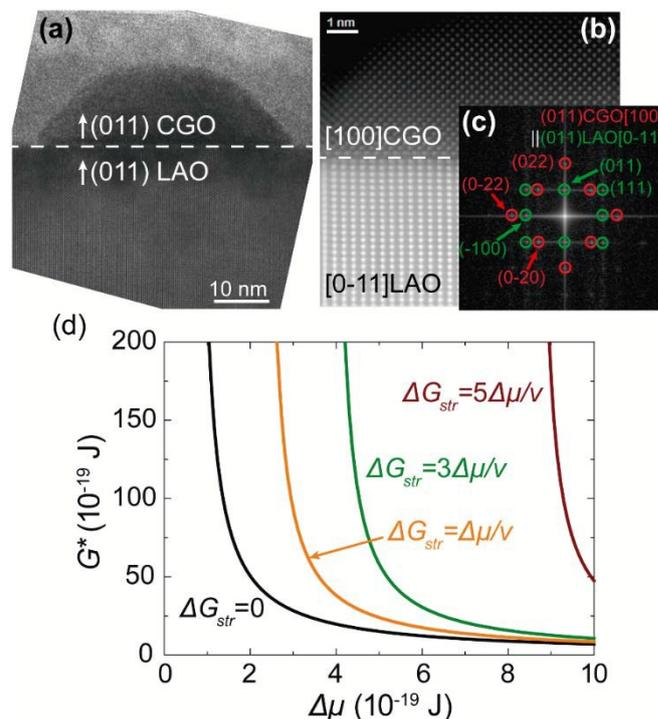
**Figure 6.** (a) HRTEM image of a short length (011)CGO island on (011)LAO. (b) HAADF-STEM characterization, and (c) power spectrum of an equivalent island viewed from the [100]CGO//[0-11]LAO zone axis. The sample was grown at 1100 °C, 20 °C s<sup>-1</sup> for 5 min in O<sub>2</sub>. (d) Dependence of the nucleation barrier ( $G^*$ ) with the supersaturation ( $\Delta\mu$ ) for different strain contributions ( $\Delta G_{str}$ ).
