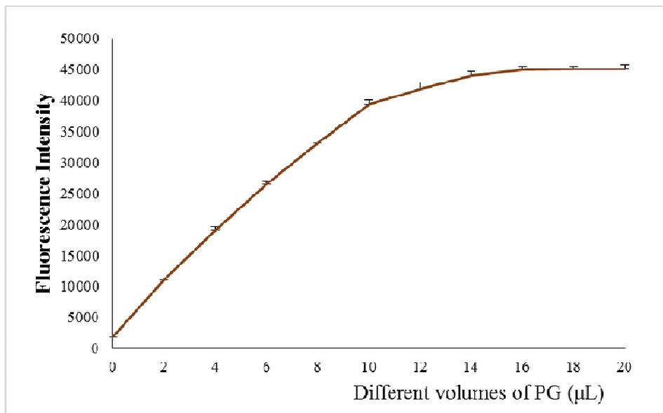
**Fig. 2.** The fluorescence intensity changes depending on the volumes (2, 4, 6, 8, 10, 12, 14, 16, 18 and 20 µL) of 10× PG solutions.
