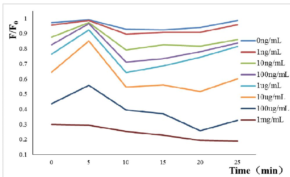
**Fig. 3.** Optimization on the reaction time of aptamer and  $\text{Pb}^{2+}$  to form a G4 structure after the addition of aptamer into  $\text{Pb}^{2+}$  of different concentrations.
