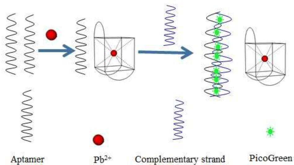
Configurations and measurement principles of label-free fluorescent aptamer-based PG assay for  $Pb^{2+}$  detection.
