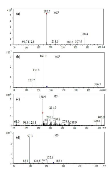
Fig. 5. LC-MS/MS Spectra (MS1 and MS2) of 3-O-methylgallic acid (a and b) and 2,6 dimethoxybenzoquinone (c and d) formed after 240 minutes of SA oxidation on PbO2 anode. japp = 15 mA cm-2; pH = 1.8; T = 30  $^{\circ}$  C.
