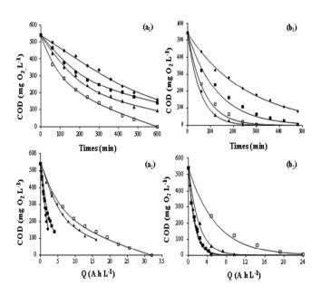
Fig. 1. Effect of current density on the variation of COD with (a1 and b1) electrolysis time and (a2 and b2) specific charge during the electrolysis of 540 mg O2 L-1 COD of SA solutions in 0.5 M H2SO4. T = 30°C; (a1 and a2): AO-PbO2; (b1 and b2): AO-BDD; japp: ( $\bullet$ ) 8; ( $\blacksquare$ ) 15; ( $\blacktriangle$ ) 60 and ( $\Box$ ) 120 mA cm-2.
