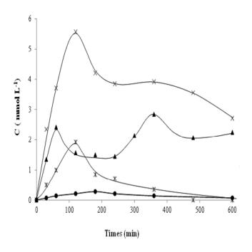
Fig. 7. Evolution of the concentration of carboxylic acids detected during the anodic oxidation of 2 mmol L-1 SA solutions in 0.5M H2SO4 on Ta/PbO2 anode. japp =15 mA cm-2; pH= 1.8; T= 30°C. ( $\bullet$ ) Maleic acid, ( $\vee$ ) Glyoxylic acid, ( $\times$ ) Formic acid and ( $\triangle$ ) Oxalic acid.
