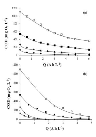
Fig. 2. COD abatement vs. specific charge time during the electrolysis of SA solutions in 0.5 M H2SO4. (a) AO-PbO2 and (b) AO-BDD. T=30 °C; japp =15 mA cm-2; Initial COD concentration: ( $\bullet$ ) 136; ( $\blacktriangle$ ) 280 ( $\blacksquare$ ) 540 and ( $\Box$ ) 1100 mg O2 L-1.
