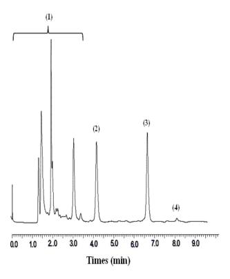
Fig. 6. HPLC chromatograms after 240 min of anodic oxidation of 2 mmol L-1 SA at Ta/PbO2 anode. japp =15 mA cm-2; pH= 1.8; T= 30°C. (1) Carboxylic acids; (2) 3-O-methylgallic acid; (3) SA; (4) 2,6 dimethoxybenzoquinone.
