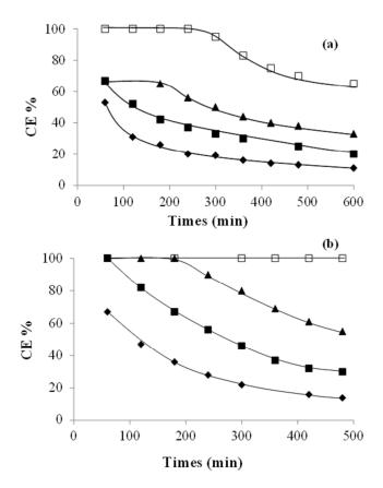
Fig. 4. Current efficiency vs. time during anodic oxidation of SA solutions on (a) Ta/PbO2 and (b) BDD anodes. T =  $30^{\circ}$ C; japp =15 mA cm-2; Initial COD concentration: (•) 136; (•) 280 (•) 540 and (□) 1100 mg O2 L-1.
