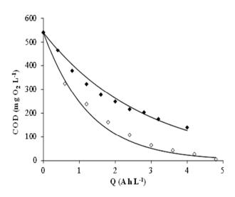
Fig. 3. Comparison of the trend of COD during anodic oxidation of SA on ( $\bullet$ ) PbO2 and ( $\diamond$ ) BDD anodes. Conditions: T=30 °C; japp =15 mA cm-2; pH = 1.8; COD0= 540 mg O2 L-1 .
