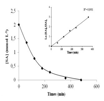
Fig. 8. SA decays with time during anodic oxidation of 2 mmol L-1 SA solution in 0.5 M H2SO4 at Ta/PbO2 anode.  $T = 30^{\circ}C$ ; japp= 15 mA cm-2. The inset panel shows its kinetic analysis assuming that the SA follows a pseudo-first-order reaction.
