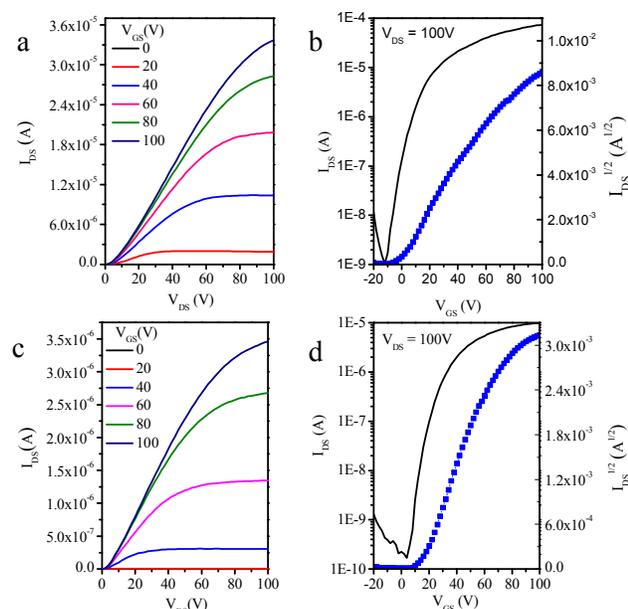
**Fig. 6** Output (a, c) and transfer (b, d) curves of an OTFT device based on a thin film of **PIDTOBT** (a, b) and **PIDTOBTz** (c, d) annealed at 200 °C
