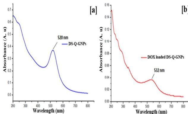
Fig. 12 UV-Visible spectra of DS-Q-GNPs and DOX loaded GNPs
