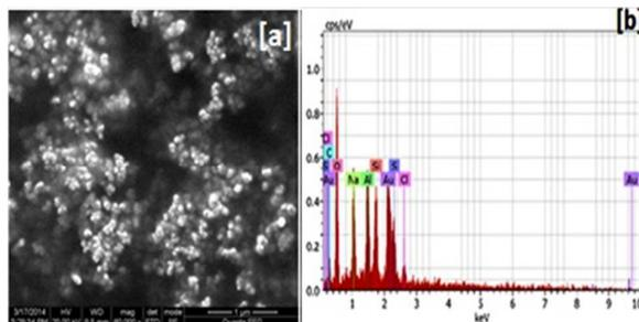
Fig. 2 (a) FE-SEM image of DS-Q-GNPs and (b) EDS spectrum of DS-Q-GNPs
