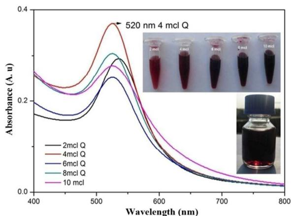
Fig. 1 UV-Visible spectra of DS-Q-GNPs
