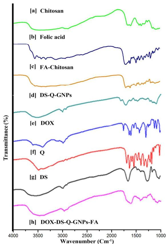
Fig. 6 GNPs FT-IR spectral analysis of (a) Chitosan, (b) Folic acid, (c) FA-Chitosan, (d) Dextran sulphat stabilized quercetin reduced GNPs; (e) Doxorubicidin; (f) Quercetin; (g) Dextral sulphate; (h) Doxorubicidin loaded Dextran sulphat stabilized quercetin reduced
