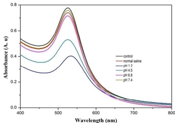
Fig. 7 *In vitro* stability showing effect of pH on DS-Q-GNPs (Mean  $\pm$  S.D; n=3)
