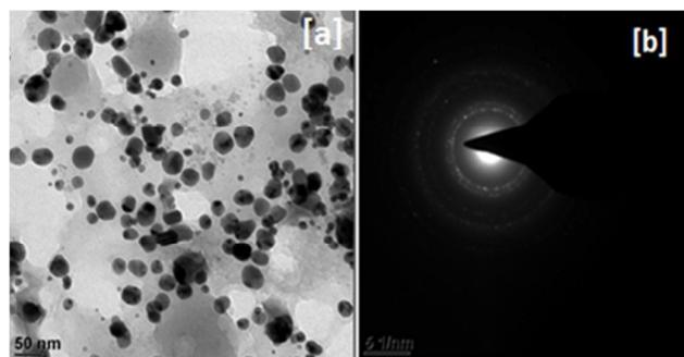
Fig. 3 (a).TEM image of DS-Q-GNPs and (b) SAED pattern of DS-Q-GNPs
