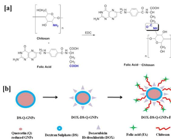
Scheme 1 Schematic representation for (a) Mechanism of folic acid-chitosan conjugation and (b) synthesis of quercetin reduced and dextran sulphate stabilized gold nanoparticles
