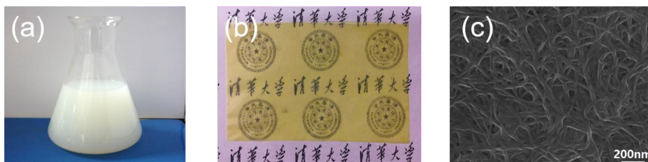
Fig. 7 Characterization of PPTA film: (a) PPTA nanofiber dispersion; (b) PPTA film; (c) SEM micrograph of PPTA membrane
