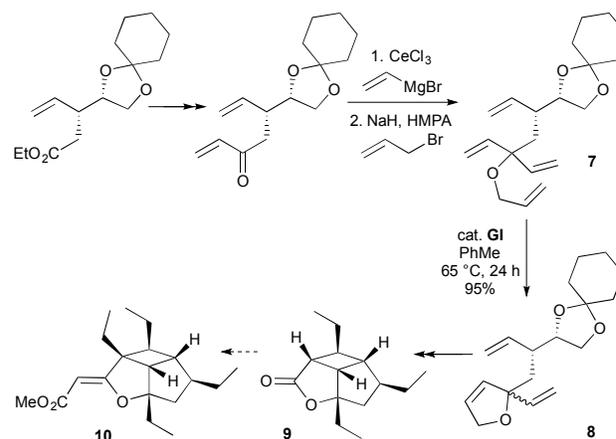
**Scheme 4** Synthesis of the core of hippolachnin A (**10**).
