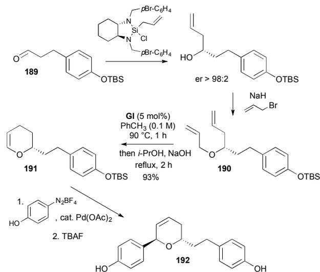
**Scheme 57** Synthesis of 5,6-dehydro-de-*O*-methyl centrolobine (**192**) using RCM-isomerisation.
