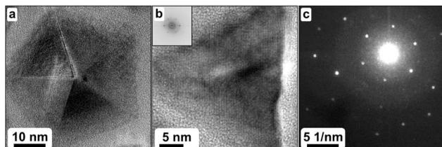
**Fig. 2.** Growth mechanism:  $\text{Fe}_{0.05}\text{Ni}_{0.95}$  precursors after a reaction time of 5 minutes. (a) HRTEM of a pentagonally twinned particle. (b) HRTEM image and (c) NED of a single-crystal flat particle displaying a hexagonal pattern with  $d$ -distances of  $2.2(1) \text{ \AA}$ .
