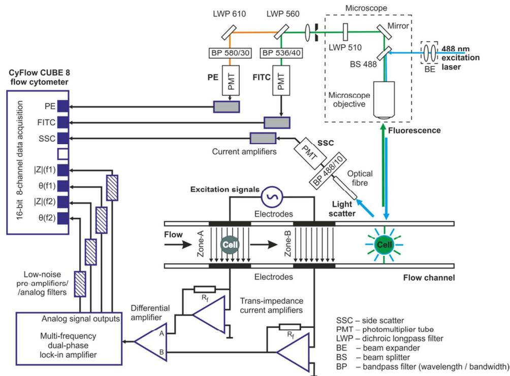
**Figure 2:** Measurement setup for combined flow cytometric optical and vector impedance measurements of blood cells and microparticles.
