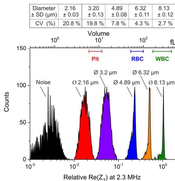
**Figure 3:** Normalized histogram (in-phase signal amplitudes) of monodisperse fluorescent calibration particles and corresponding coefficients of variations (CV) measured with the  $\mu$ FCM at a frequency of 2.3 MHz. Fluorescence was detected in the FITC channel and applied for colour gating of the particles. The suspension contained custom manufactured polystyrene beads (PS-FluoGreen, Microparticles GmbH, Germany). The driving voltage amplitude was set to its maximum value of 750 mV.
