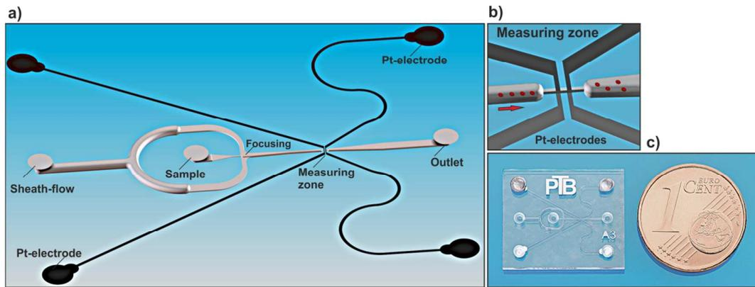
**Figure 1:** (a) Design of the flow channels and electrodes of the  $\mu\text{FCM}$ . (b) Close-up of the measuring zone. (c) Photo of the  $\mu\text{FCM}$  device showing proportions.
