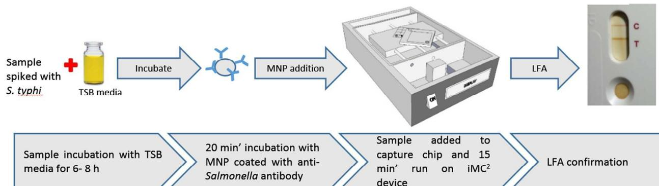
An affordable immuno-magnetic cell capture system for bacterial detection in 7 hours with 10 CFU/ml sensitivity.
