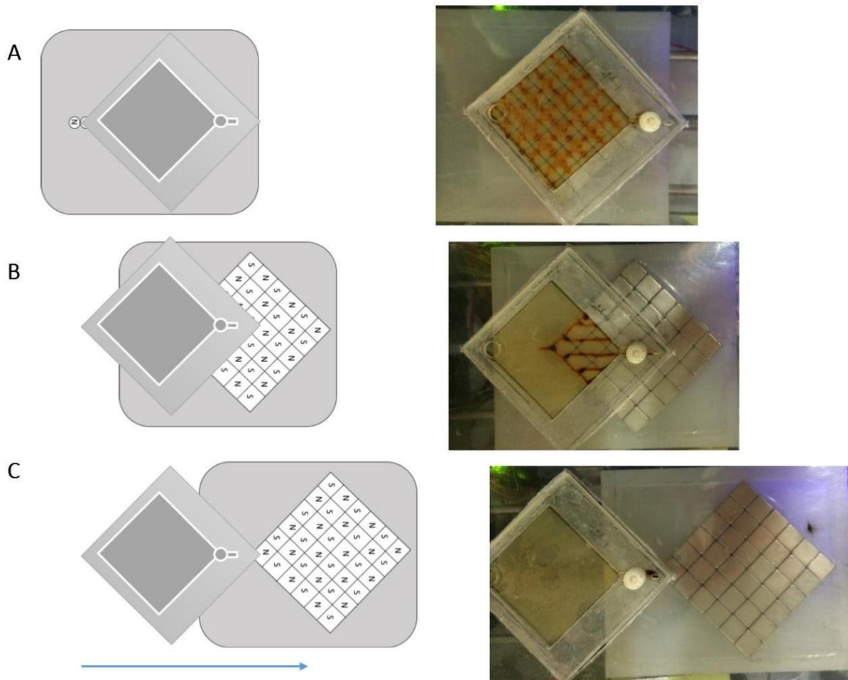
**Figure 3:** Time-lapsed images of immunomagnetic enrichment process by displacement of the magnetic cassette. **(A)** After 5 min: Cells collected at the highest magnetic field gradients near the bottom surface. **(B)** After 10min: Sweeping action on the MNP-Ab cell complexes as the magnetic field is moved in small steps using a linear positioner. **(C)** After 15 min: Cells concentrated into the 50 µl volume recovery chamber allowing for 100× enrichment.
