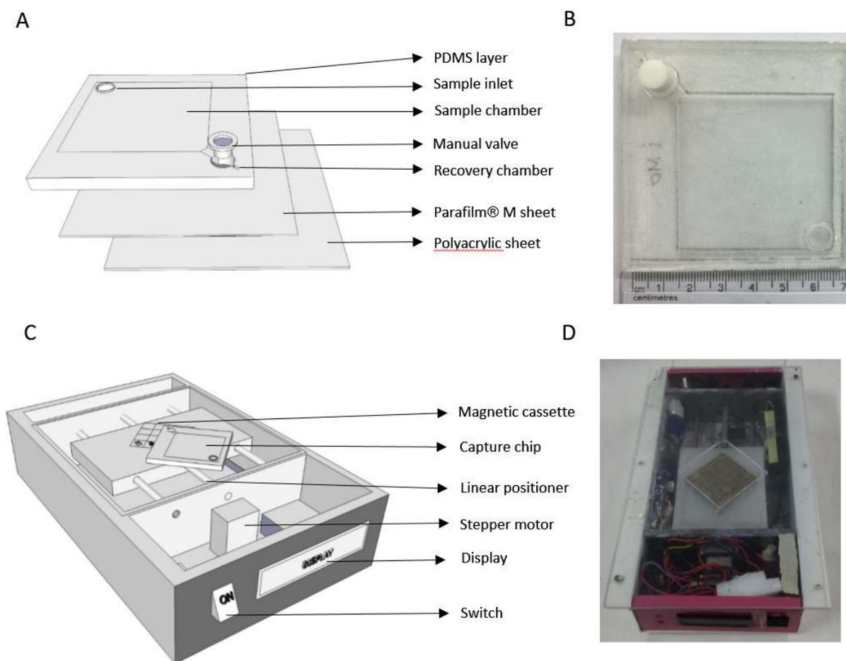
**Figure 1:** (A) Schematic representation of the capture chip designed to hold and process the MNP-Ab labeled samples. Capture chip is made of 3 layers: (i) *Top*: mold-crafted PDMS layer with
