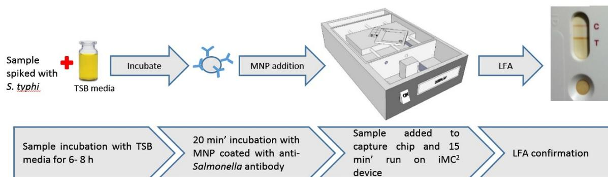
**Figure 2:** Overall schematic of the immunomagnetic capture enrichment of *Salmonella* cells using the iMC<sup>2</sup> system and result confirmation using an LFA.
