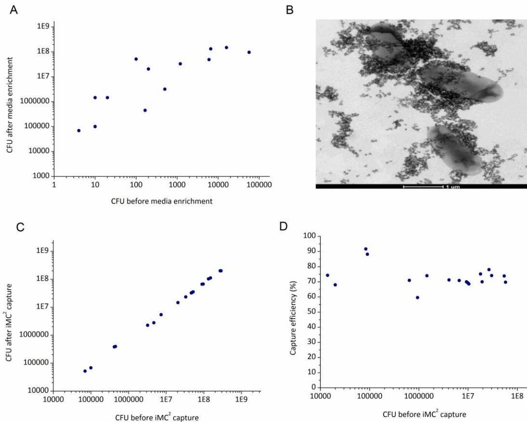
**Figure 4:** Performance characterization of iMC<sup>2</sup> device with spiked buffer sample: **(A)** Plot of the *S.typhi* counts before and after 8 h incubation in TSB media. **(B)** TEM image of the MNP-bound *S.typhi*. **(C)** Plot of *S.typhi* concentration prior to and after processing with the iMC<sup>2</sup> device. **(D)** Capture efficiency of device calculated by comparing cell count before and after immunomagnetic enrichment.
