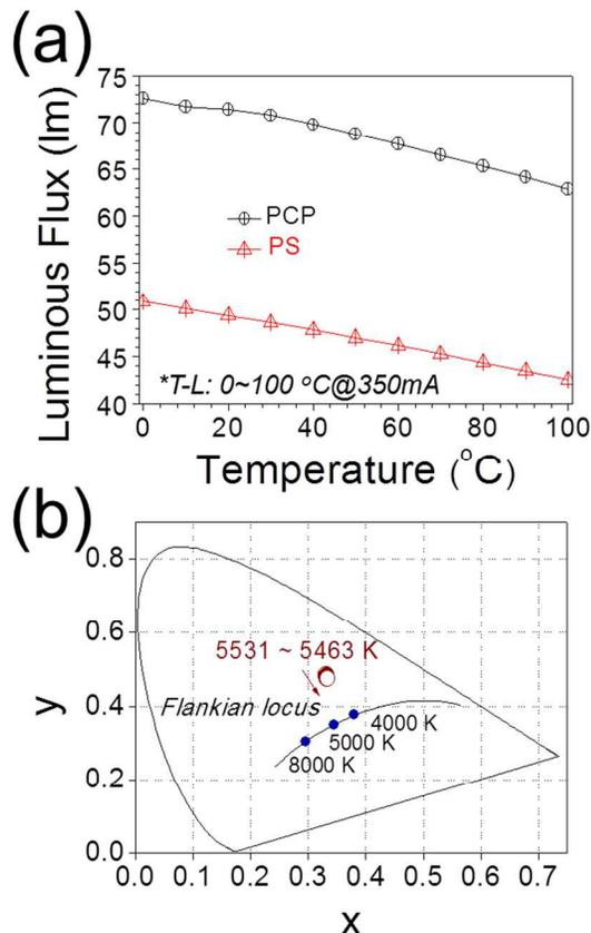
**Figure 4.** (a) T-L spectra of the PCP compared with PS. (b) CIE colour coordinates of PCP on blue LEDs
