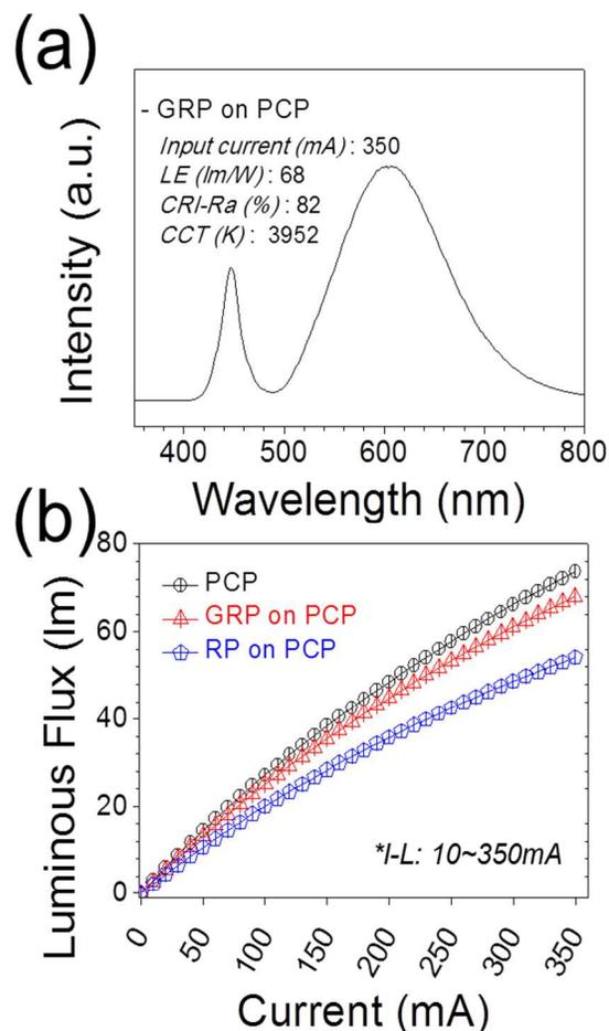
**Figure 6.** (a) EL spectrum of the fabricated samples. (b) I-L spectra of the fabricated samples
