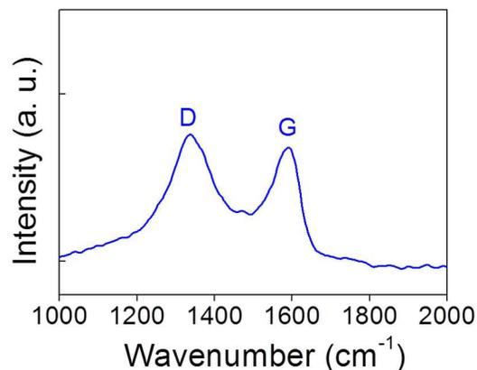
**Figure 5.** Raman spectrum of rGO.
