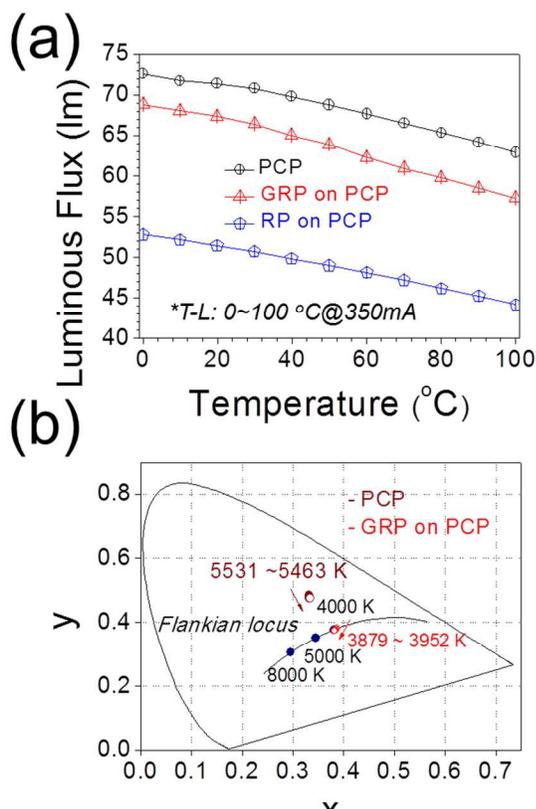
**Figure 7.** (a) T-L spectra of GPL on PCP. (b) CIE colour coordinates of PCPs on blue LEDs.
