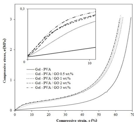
**Fig. 8** Graphical representation illustrating the mechanical response of Gel - PVA and Gel - PVA / GO spongy composites against compressive stress.
