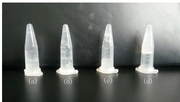
Fig. 2. The apparent gel-forming properties of (a) 1.4 wt% XG, (b) 0.35 wt % XG-SA, (c) 0.7 wt % XG-SA and (d) 1.4 wt % XG-SA in water.
