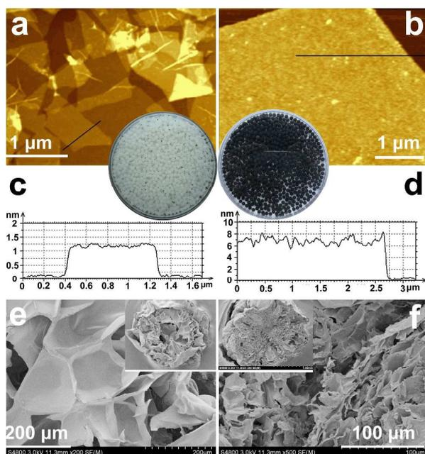
**Fig. 2** Tapping mode AFM images of CRGO (a) and CRGO-GOD (b). The height profile of the AFM images of CRGO (c) and of CRGO-GOD (d). SEM images of the section GOD@Alg (e) and CRGO-GOD@Alg (f) beads dried in a freezer dryer.
