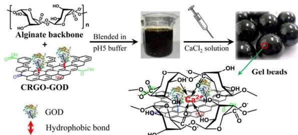
**Scheme 1** Schematic representation of the synthesis of CRGO-GOD@Alg beads.
