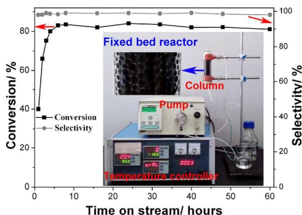
**Fig. 5** The conversion and selectivity of fixed-bed reaction and the photograph of fixed-bed reactor (inset).
