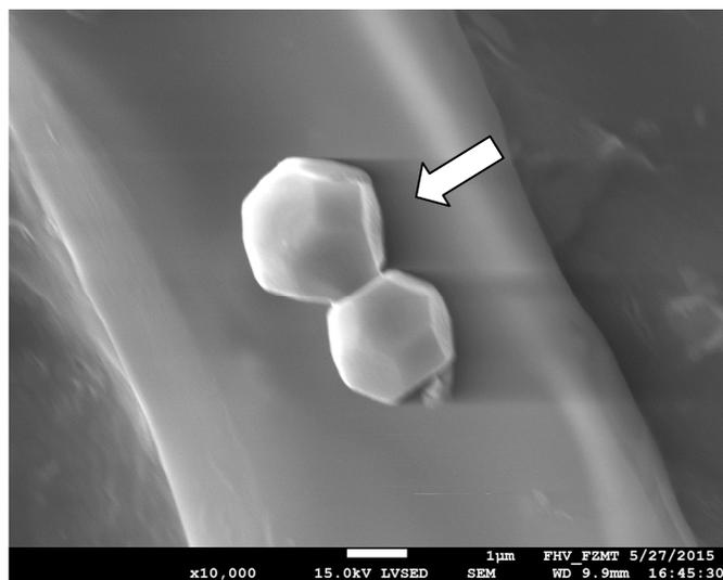
Fig.3 Electron micrographs of  $\text{Cu}_2\text{O}$ /binder treated sample A and EDX analysis (arrow indicates  $\text{Cu}_2\text{O}$  particle)
