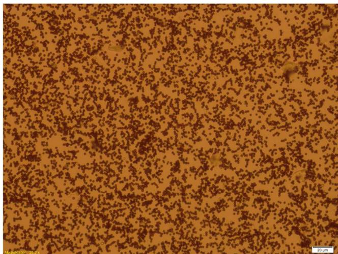
Fig. 1 Light microscope images of Cu<sub>2</sub>O microparticles
