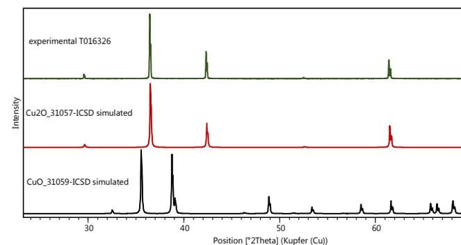
Fig. 2 Comparison of the experimental XRD pattern of Cu<sub>2</sub>O particles (TO16326) with the simulated pattern of Cu<sub>2</sub>O and CuO
