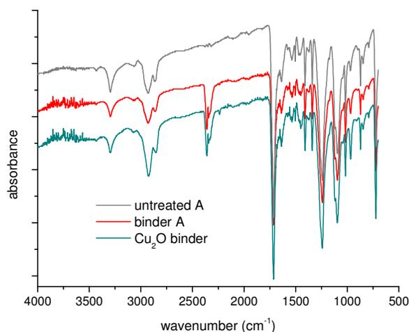
Fig. 5 FTIR-ATR spectra of untreated sample A, sample with binder alone and Cu<sub>2</sub>O and binder treated sample
