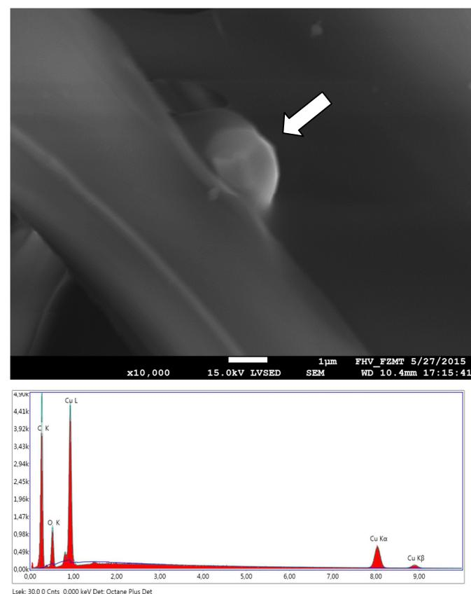
Fig.4 Electron micrographs of 10 x washed  $\text{Cu}_2\text{O}$ /binder treated sample A and EDX analysis (arrow indicates  $\text{Cu}_2\text{O}$  particle)
